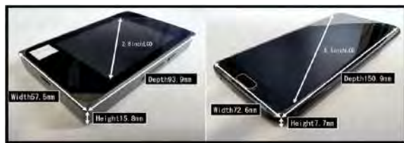
Fig. 2. Appearance of the BL-02 IoT device for business use and the GalaxyS7-edge smartphone for general use.
