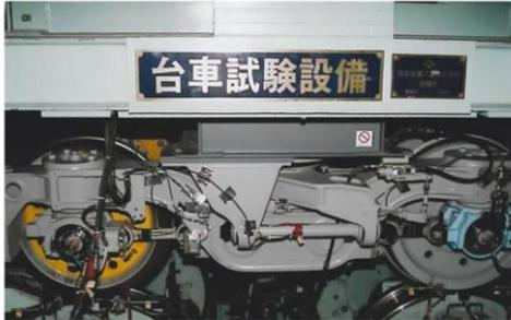
Photo 1 Bogie test stand and test bogie.
