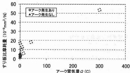
Fig.2 Effect of arc discharge on wear of carbon based contact
