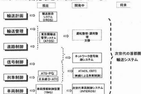
Fig.1 Example of System Related to Railway Operation
