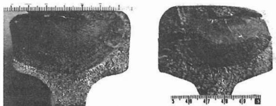
(a) Rail squats (b) Gauge corner cracking
