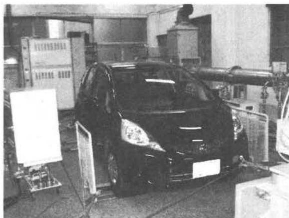
Fig.2 Test on Chassis Dynamometer
