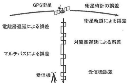
Fig.7 Six elements cause GPS error
