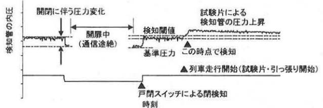
Fig.14 Behavior of the tube sensor and time history of pressure by closes or tape
