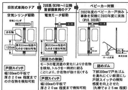
Fig1. Transition of door engine and door-catch-switch (JR-East)
