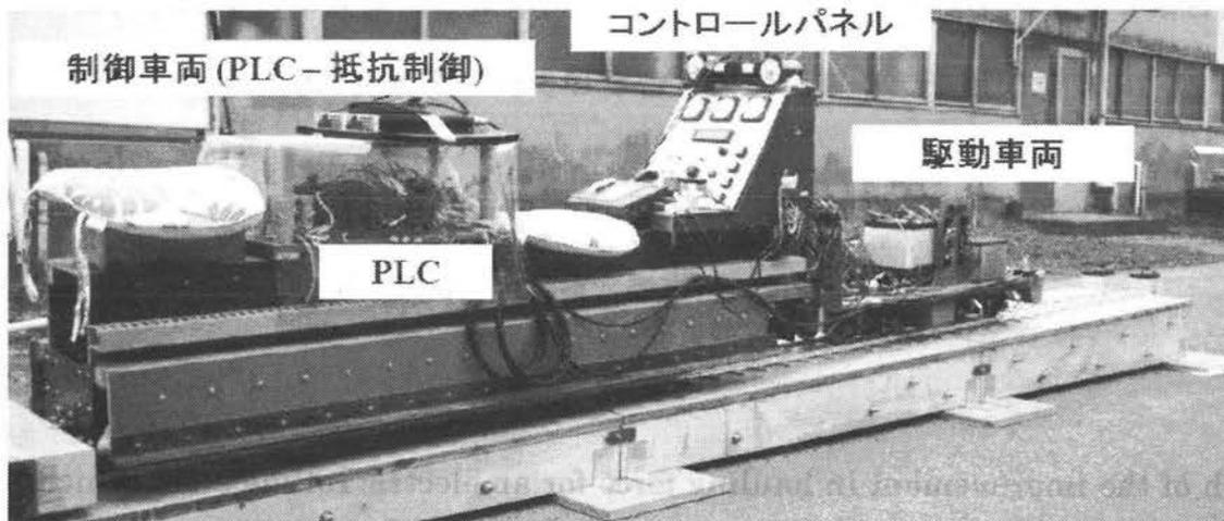
Fig2.1 1/8.4scale test model of electric rolling stock
