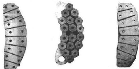
a) Existing lining      b) Isolation Pressure pad      c) Resin lining
