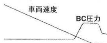
Fig. 9 Character of the braking noise (Shoe head which was made to become dented)
