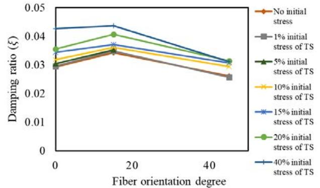
Fig.9 The first-mode flexural damping ratio variation with fiber orientation degree.
