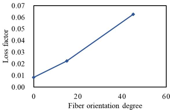
**Fig.5** Variation of loss factor with fiber orientation degree
