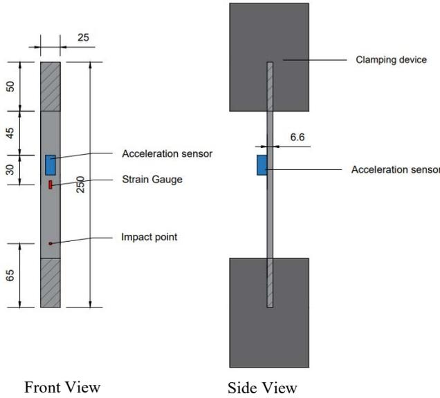
**Fig.2** Specimen dimension and experimental setup.
