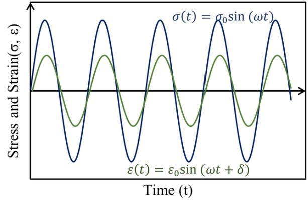
Fig.1 Stress and strain curves in the time domain.
