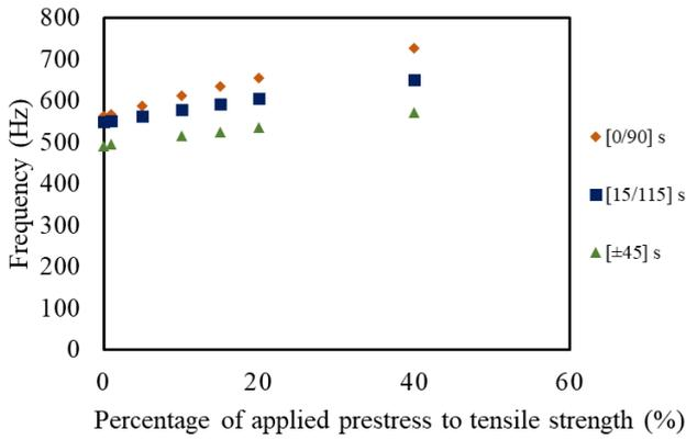
Fig.6 The variation of the first-mode flexural frequency with initially applied stress.
