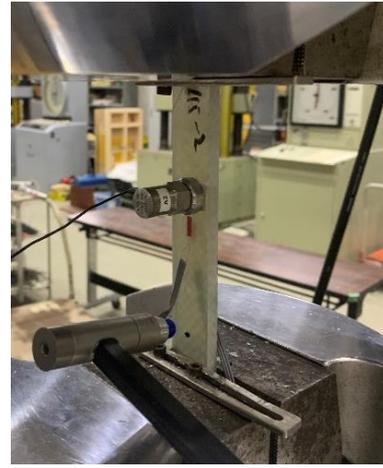
**Fig.3** Impact test.
