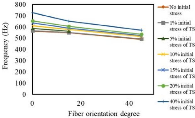
Fig.7 The variation of the first-mode flexural frequency with fiber orientation degree.
