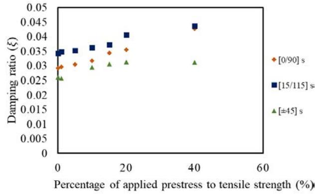
Fig.8 The first-mode flexural damping ratio variation with initially applied stress.
