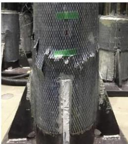
図-4 圧縮側CFRP圧壊
