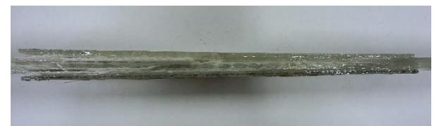
(e) D200-DD (補修板剥離)
