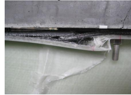
(b) HFRP flange delamination failure
