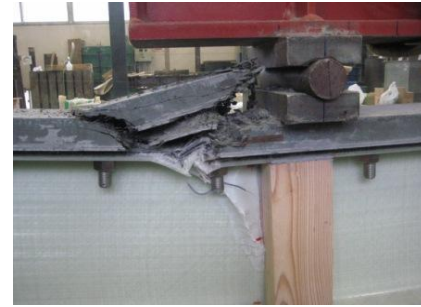
(a) Crushing of UHSFRC slab
