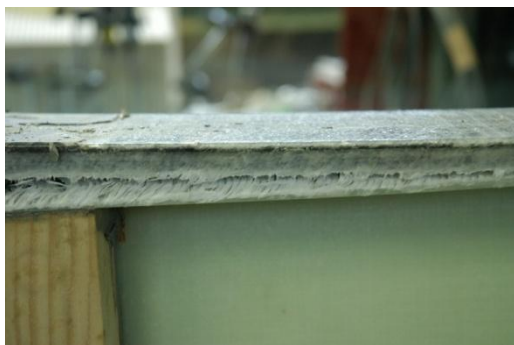
Fig. 7 Closer view of delamination
