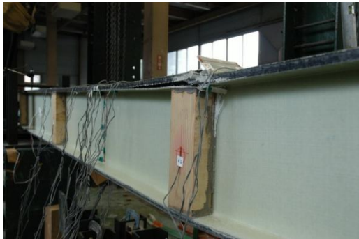
Fig. 6 Crushing of fibers and delamination
