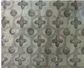
Fig.2 Punching metal shapes: (i) cross and round (Left); (ii) oblong (Right)
