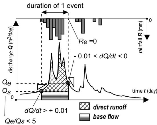
**Fig-6** Conceptual representation of extracting unit hydrograph
