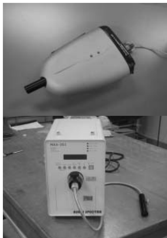
図-5 Field Spec Hand Held と High Power キセノン光源 MAX-301
