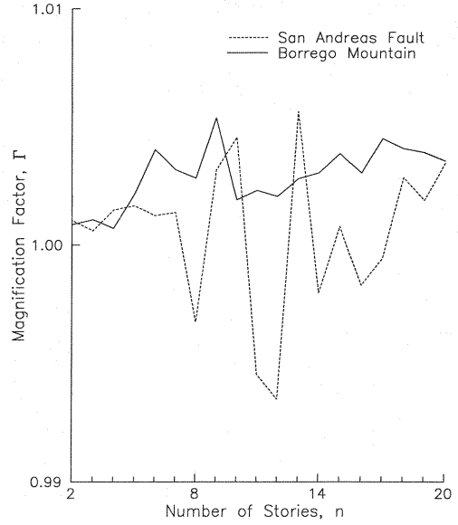
Fig.9 Effect of Concentration of Energy in Long Period Waves on Rocking Contributions at Pasadena Site.
