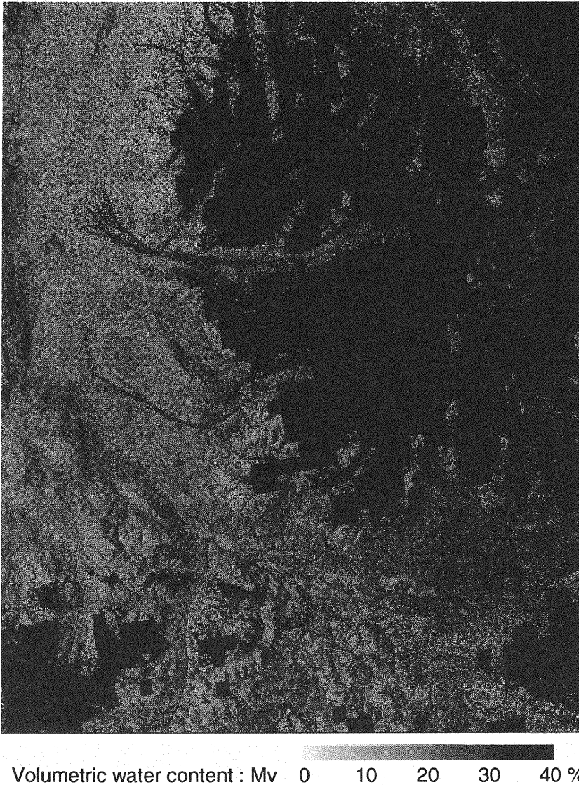
Fig. 7 50m mesh soil moisture map of the Tibetan Plateau by JERS-1 SAR image (Aug. 17, 1993)
