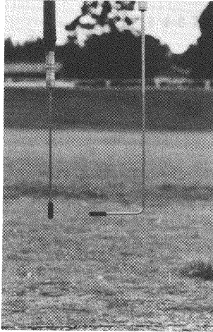
Photo 1 Probes of electromagnetic anemometers
