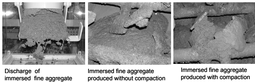
Photo 3 Discharge of immersed fine aggregate from the batcher
