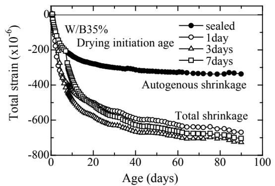
**Fig.6** Time-dependent change in total shrinkage strain (W/B35%)
