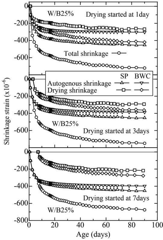
Fig.15 Components of shrinkage (W/B25%)
