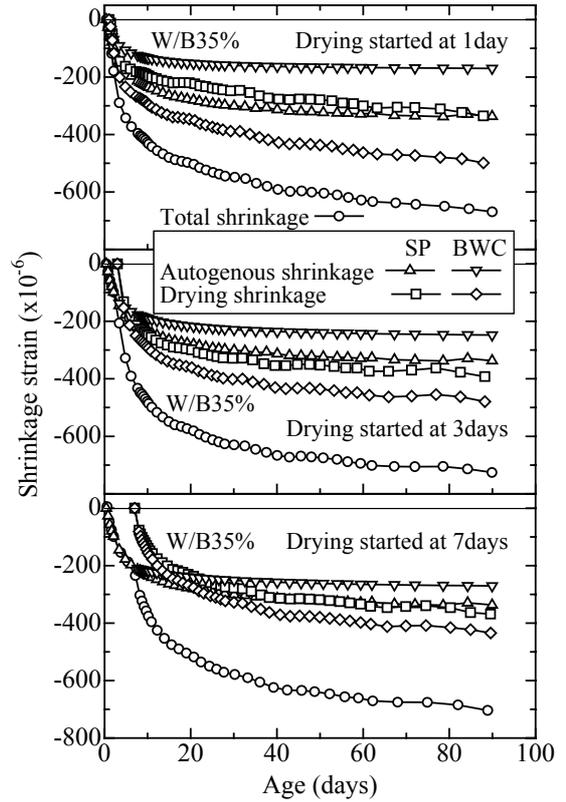
Fig.16 Components of shrinkage (W/B35%)
