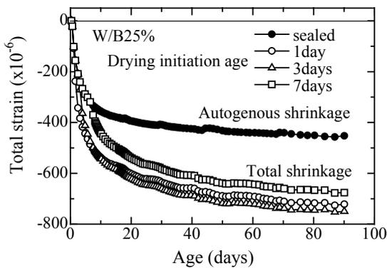
**Fig.5** Time-dependent change in total shrinkage strain (W/B25%)
