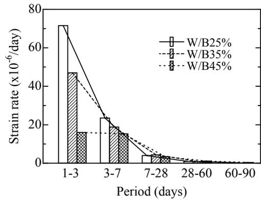
**Fig.4** Comparison of strain rate
