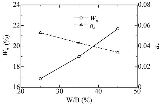
**Fig.11** Influence of W/B on  $W_n$  and  $a_s$  under sealing
