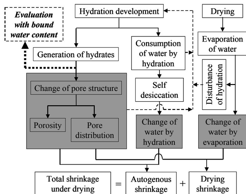
Fig.1 Relation between autogenous shrinkage and bound water content
