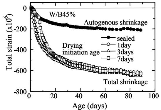
**Fig.7** Time-dependent change in total shrinkage strain (W/B45%)
