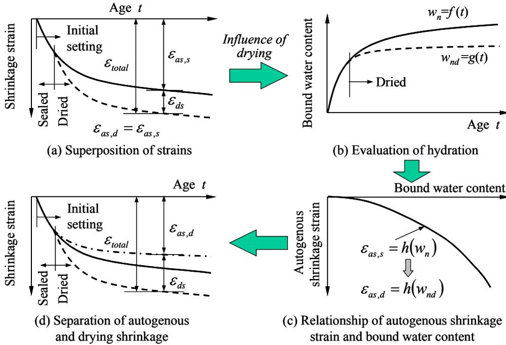
**Fig.2** Approach to evaluating autogenous shrinkage under drying and drying shrinkage
