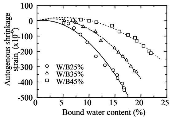
**Fig.14** Relationship of autogenous shrinkage strain and bound water content
