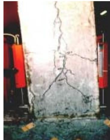
**Figure 5** Load-displacement curve and crack pattern of column 4
