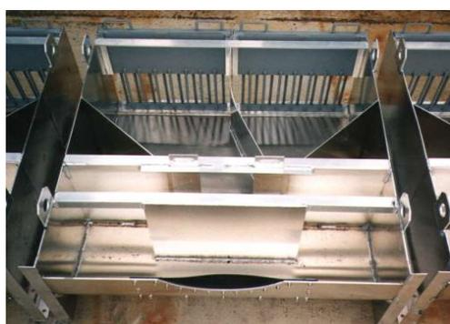
**Photo 5** Testing Apparatus with Barrier for Self-Compactability Evaluation
