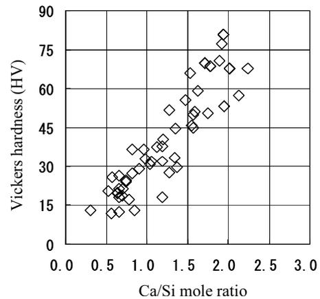
**Figure 9** Relationship between Vickers hardness and Ca/Si molar ratio of the bulk concrete
