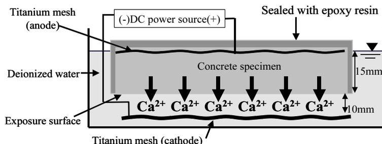
**Figure 3** Outline of electrochemical accelerated test
