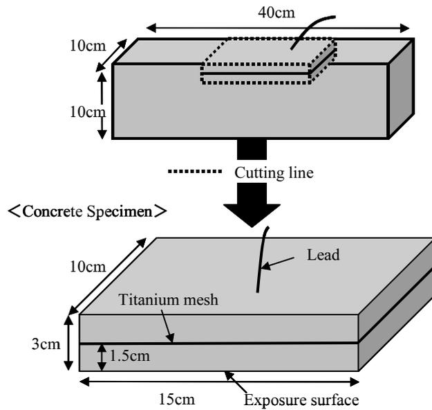
\*Specimen was sealed with epoxy resin, except on the exposure surface.
