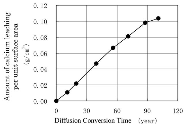
**Figure 6** Relationship between DCT and amount of calcium leaching per unit surface area
