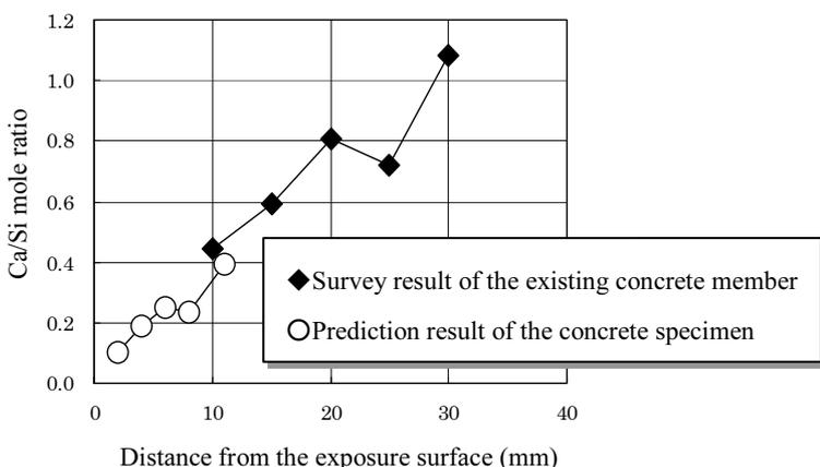
**Figure 8** Relationship between Ca/Si molar ratio of concrete specimen and existing concrete member and distance from exposure surface
