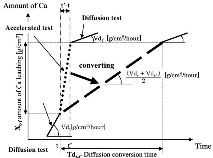
**Figure 4** Method of calculating Diffusion Conversion Time (DCT)
