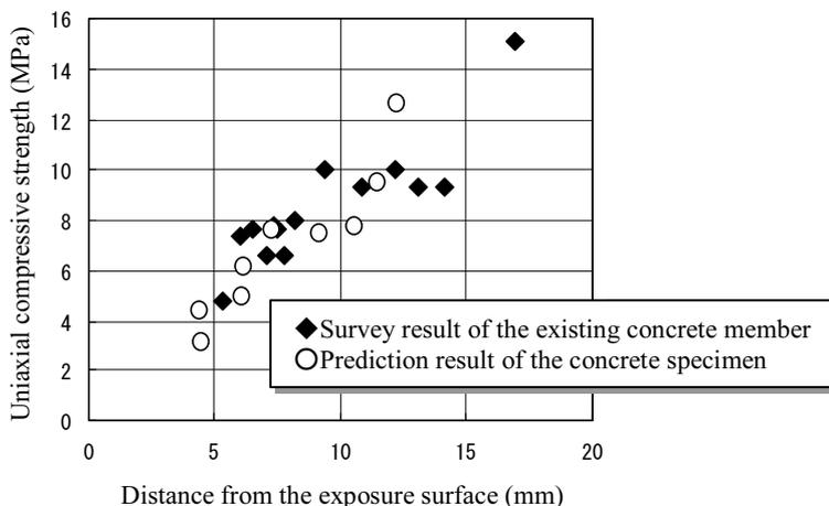
**Figure 7** Relationship between uniaxial compressive strength of concrete and distance from exposure surface
