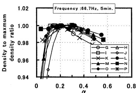
Fig.6 Dry density to maximum dry density ratio versus  $\alpha$
