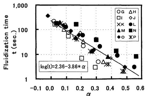
Fig.19  $\alpha$  versus fluidization time
