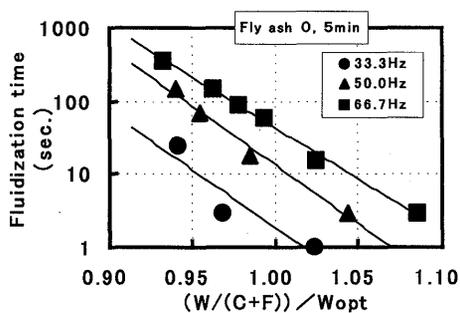
Fig.17 Fluidization time versus  $(W/(C+F)) / W_{opt}$
