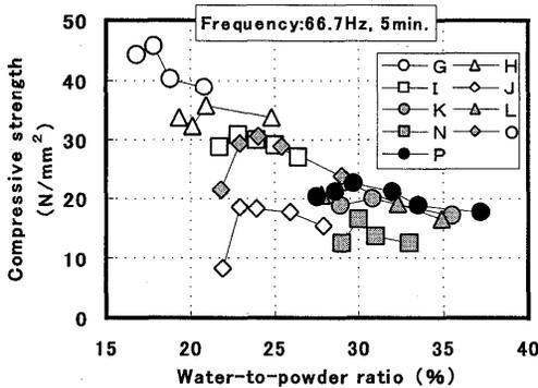
Fig.1 Compressive strength versus water-to-powder ratio
