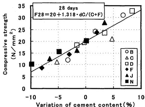
**Fig.12** Compressive strength versus variation of cement content
