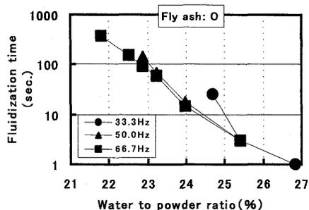
Fig.15 Fluidization time versus water-to-powder ratio
