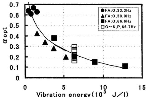
Fig.9  $\alpha_{opt}$  versus vibrarion energy
