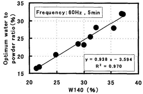
Fig.3 Optimum water-to-powder ratio versus W140
