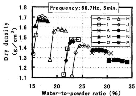
Fig.5 Dry density versus water-to-powder ratio
