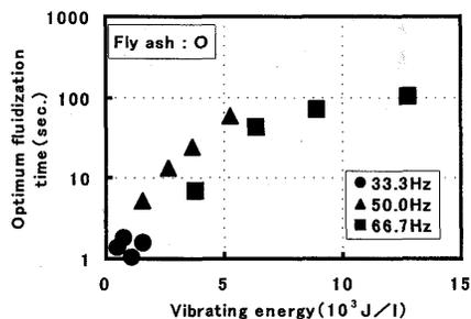
Fig.18 Optimum fluidization time versus vibration energy
