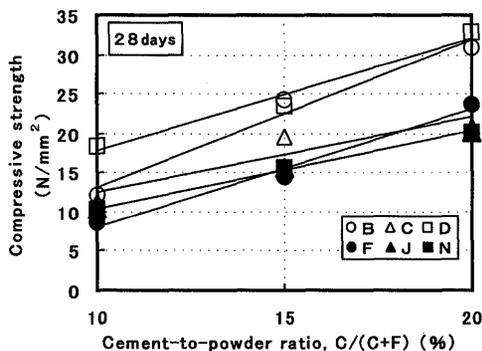
**Fig.11** Compressive strength versus cement-to-powder ratio
