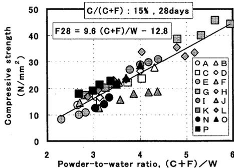
Fig.10 Compressive strength versus powder-to-water ratio
