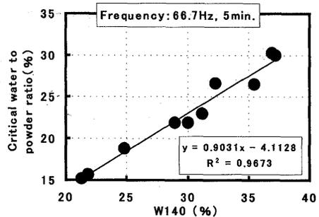
Fig.4 Critical water-to-powder ratio versus W140
