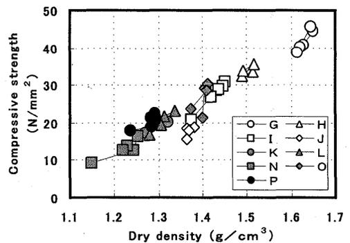
Fig.2 Compressive strength versus dry density
