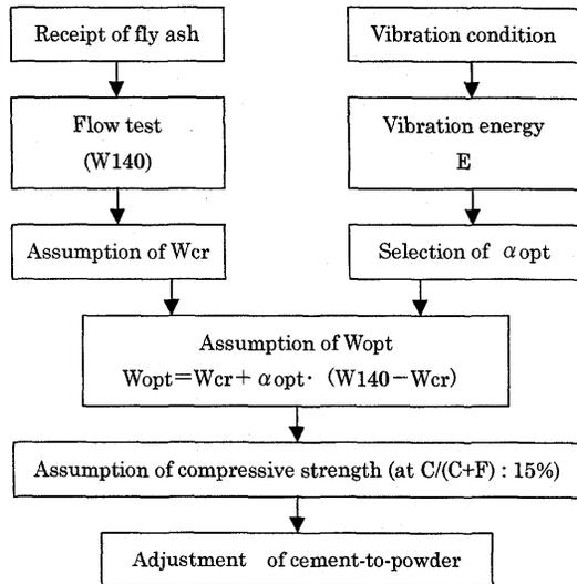
**Fig.13 Flow for selection of mix proportion**
