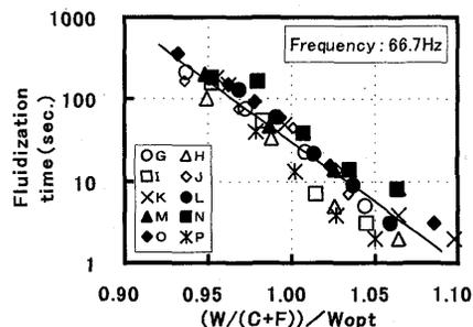
**Fig.14 Fluidization time versus (W/(C+F)) / Wopt**
