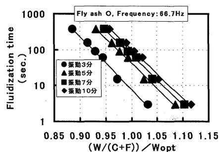
Fig.16 Fluidization time versus  $(W/(C+F)) / W_{opt}$
