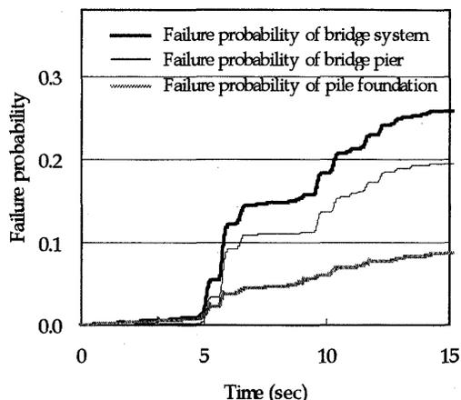
Figure 17. Failure Probability of Bridge System and its Components when Equipped with elastomeric Bearings
