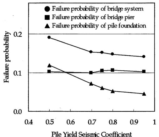
Figure 14. Relationship of Pile's Yield Seismic Coefficient to Failure Probabilities of Bridge System and with its Components
