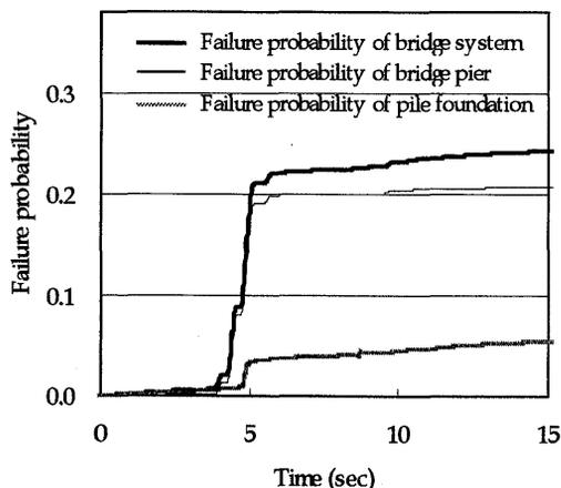
Figure 16. Failure Probability of Bridge System and its Components When Equipped with Seismic Isolation Bearings
