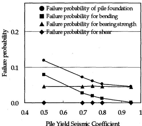
Figure 15. Relationship of Pile's Yield Seismic Coefficient to Failure Probability in Ultimate Limit State of Pile Foundation
