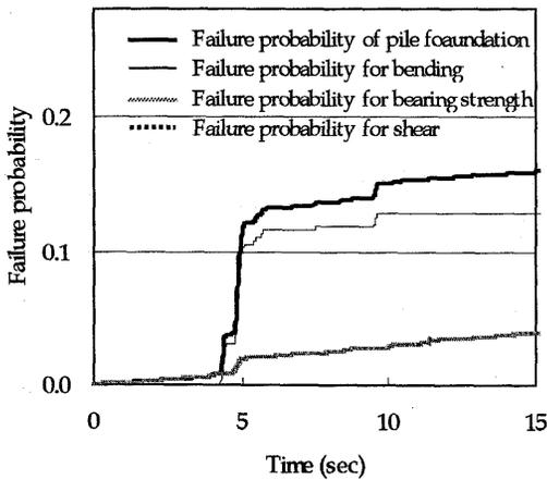
Figure 10. Failure Probability at Ultimate Limit State of Pile Foundation at Pile Yield Seismic Coefficient of 0.50
