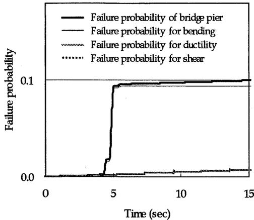
Figure 12. Failure Probability at Ultimate Limit State of Bridge Pier at Pile Yield Seismic Coefficient of 0.95
