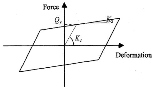
Figure 7. Bilinear Model of the Seismic Isolation Bearings
