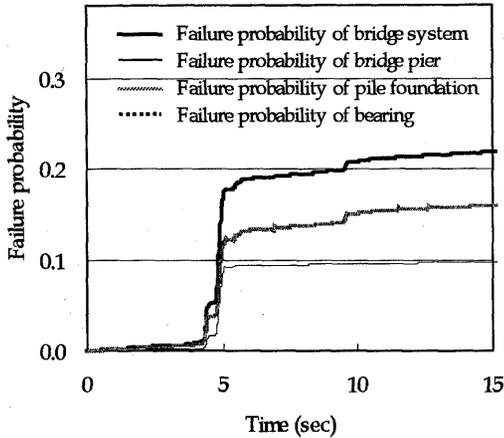
Figure 8. Failure Probability of Bridge System and its Components at Pile Yield Seismic Coefficient of 0.50
