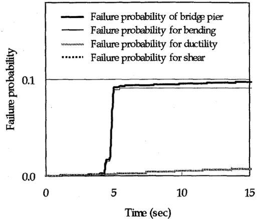
Figure 9. Failure Probability at Ultimate Limit State of Bridge Pier at Pile Yield Seismic Coefficient of 0.50
