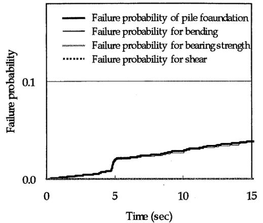
Figure 13. Failure Probability at Ultimate Limit State of Pile Foundation at Pile Yield Seismic Coefficient of 0.95
