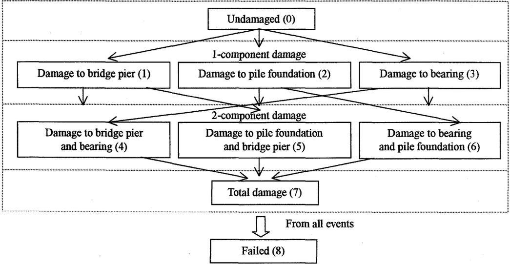
Figure 3. Damage Change Model of Bridge Analyzed
