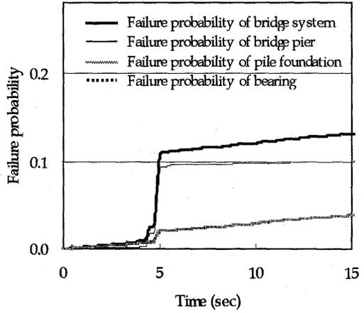
Figure 11. Failure Probability of Bridge System and its Components at a Pile Yield Seismic Coefficient of 0.95
