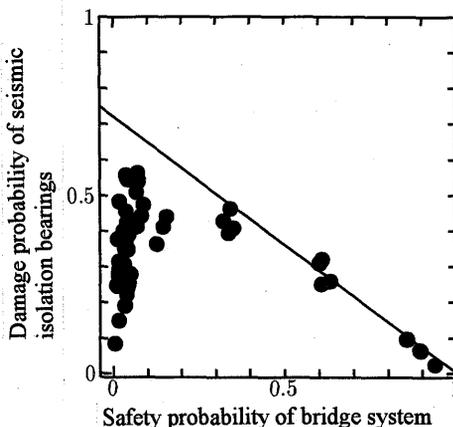
Figure 18. Bridge System Safety Probability versus Seismic Isolation Bearing Damage Probability Relationship
