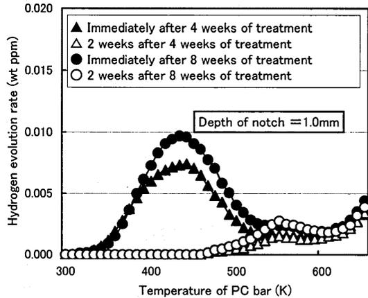
Fig.6 Hydrogen evolution curves after desalination
