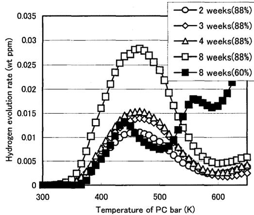
Fig.8 Hydrogen evolution curves of high-tensioned PC bar
