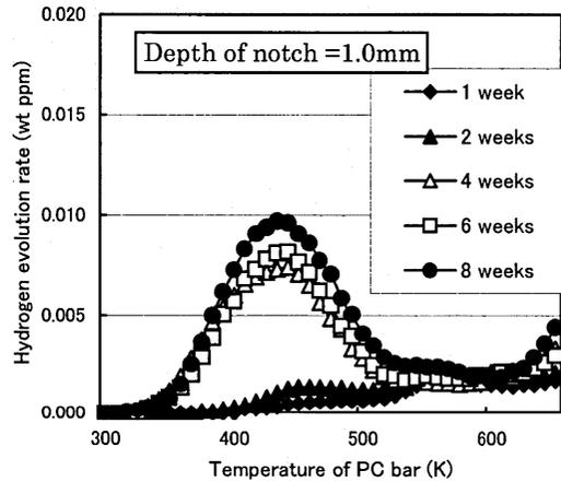
Fig.5 Hydrogen evolution curves for various treatment times
