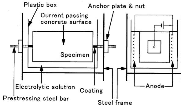
**Fig.2** Specimen and experimental set-up for desalination
