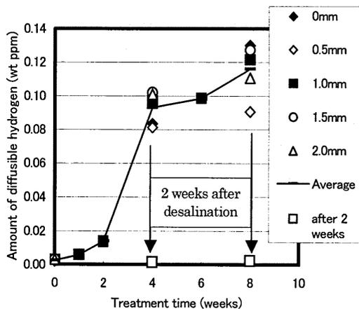
Fig.7 Relationship between diffusible hydrogen and duration of treatment
