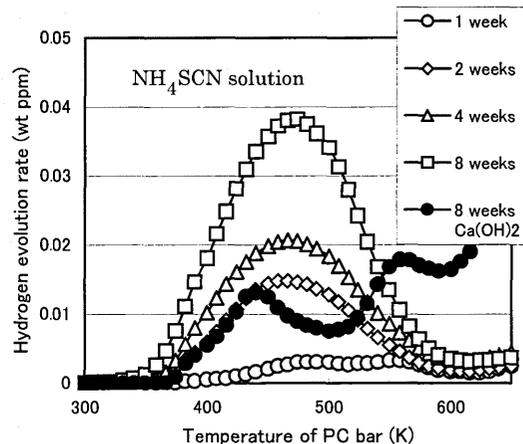
Fig.10 Hydrogen evolution curves ( $\text{NH}_4\text{SCN}$  solution)
