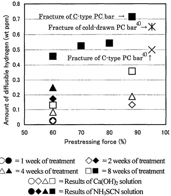
Fig.12 Relationship between prestressing force and diffusible hydrogen
