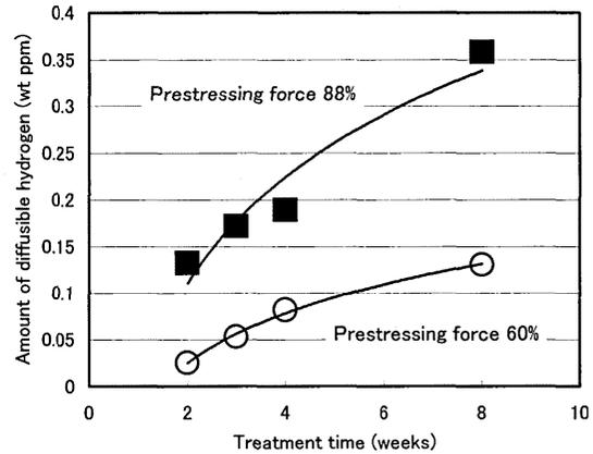
Fig.9 Relationship between diffusible hydrogen and treatment time
