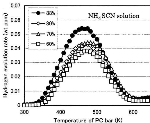
Fig.11 Hydrogen evolution curves of high-tensioned PC bar
