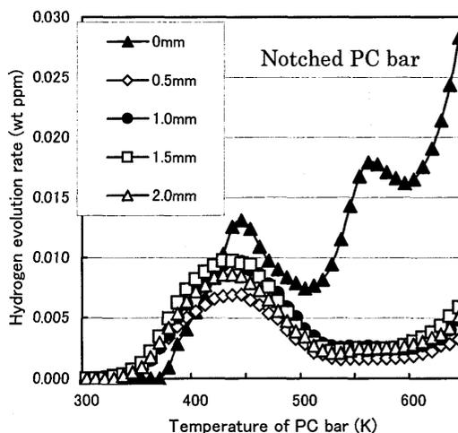
**Fig.4** Hydrogen evolution curves just after desalination
