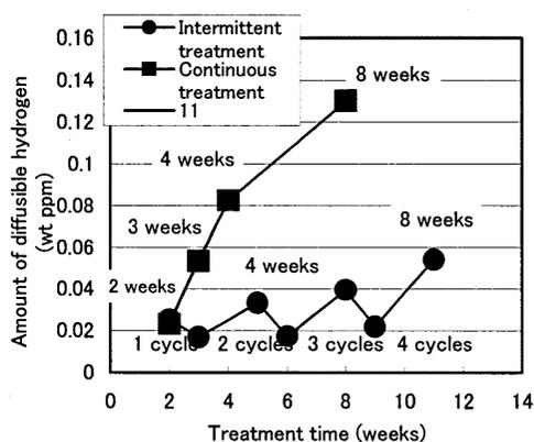
Fig.15 Relationship between treatment method and diffusible hydrogen
