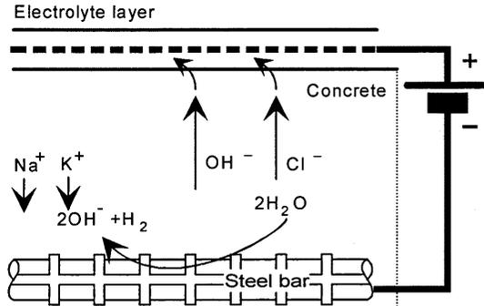
Fig.1 Mechanism of desalination
