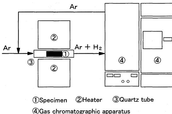
**Fig.3** Schematic diagram of hydrogen thermal analysis
