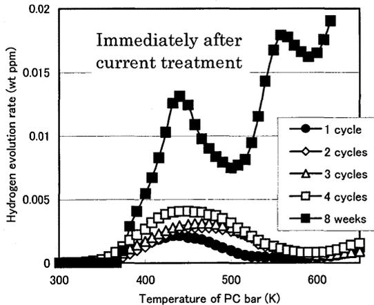
Fig.13 Hydrogen evolution curves immediately after current treatment
