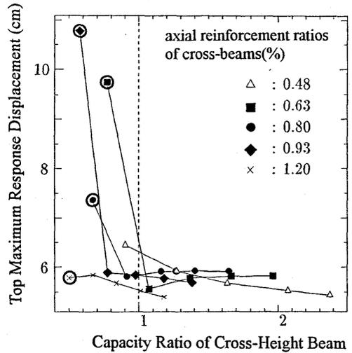
Figure 5. Top Maximum Response Displacement-Capacity Ratio Relationship of Cross-Beam
