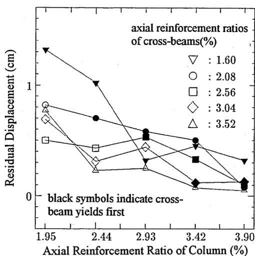
Figure 7. Reinforcement Ratio-Residual Displacement Relationship of Member
