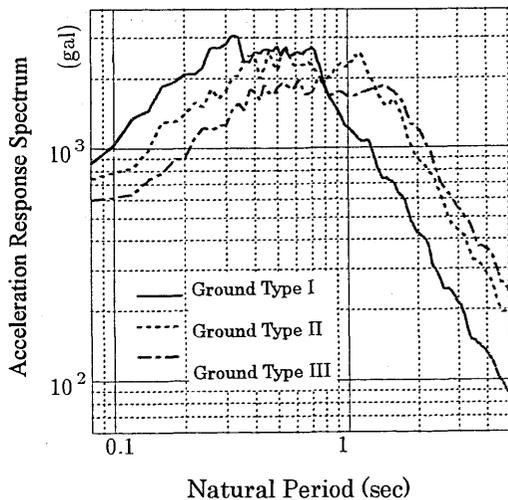
Figure 10. Acceleration Response Spectrum of Type-II Earthquake Motion
