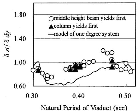
Figure 13. Comparison of Static Analysis and Dynamic Analysis (Ground Type III)
