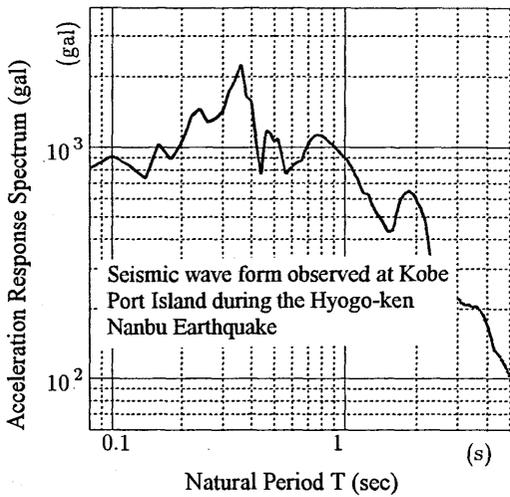
Figure 4. Acceleration Response Spectrum of Input Earthquake Motion
