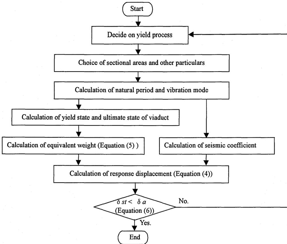
Figure 15. RC 2-story Rigid-Frame Viaduct Seismic Design Flow Chart
