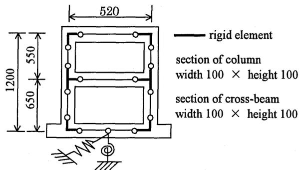
Figure 1. Viaduct Model unit: cm
