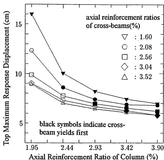
Figure 6. Reinforcement Ratio-Top Maximum Response Displacement Relationship of Cross-beam
