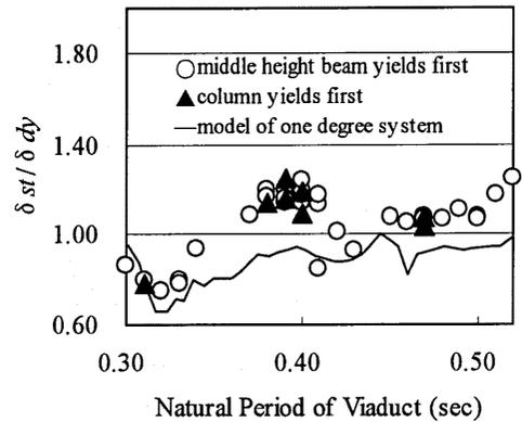
Figure 12. Comparison of Static Analysis and Dynamic Analysis (Ground Type II)
