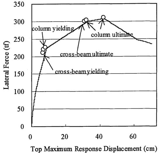
Figure 8. Example of Lateral Force of Viaduct-top Lateral Displacement Relationship
