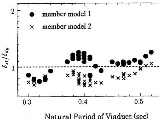
Figure 14. Comparison of Estimation Precision of Response Displacement with Different Member Models
