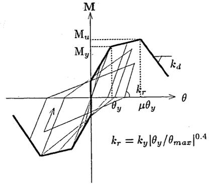
Figure 3. Bending Moment-Rotation Angle Relationship
