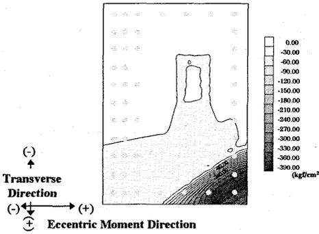
Fig. 18.3 Concrete Stress at  $+2 \delta y (2)$
