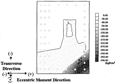
Fig. 18.5 Concrete Stress at  $+2 \delta y (3)$
