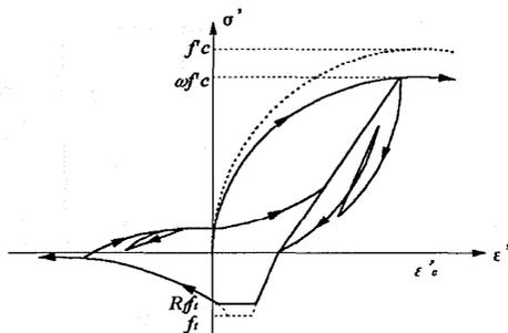
Fig. 7 Concrete Material Model [16][17]
