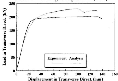
Fig. 6 Load – Displ. Relationship in the Eccentric Direction (after Damage)
