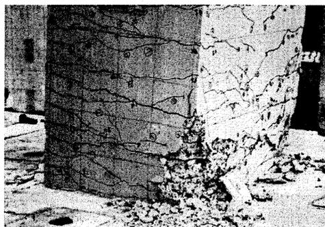
Photo 2 Damage to Specimen (base)
