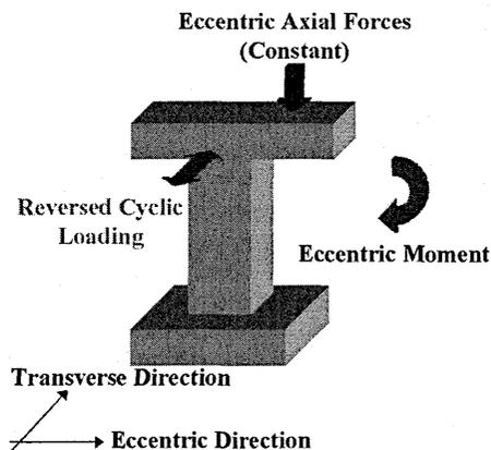
Fig. 1 Loading Direction
