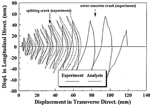
Fig. 5.1 Displ. in the Orthogonal Direct. - Dipl. in the Eccentric Direct. Relationship
