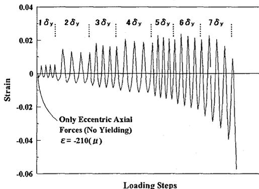
Fig.17.2 Steel Strain History of Point b
