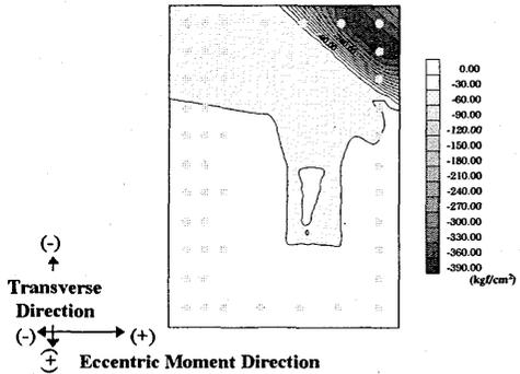
Fig. 18.8 Concrete Stress at  $-2 \delta y (4)$
