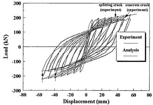
Fig.4 Load-Displacement Relationship in the Transverse Direction
