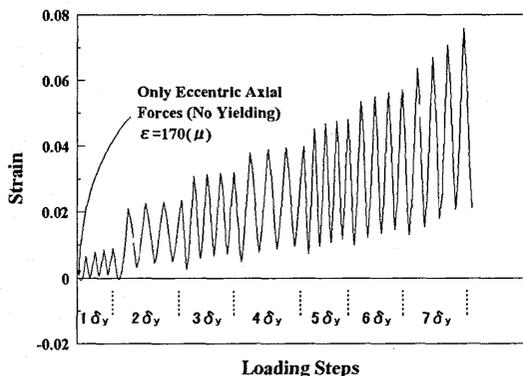
Fig.17.1 Steel Strain History of Point a
