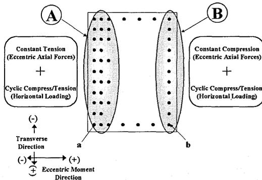
Fig.16 Re-bar Groups at Cross Section
