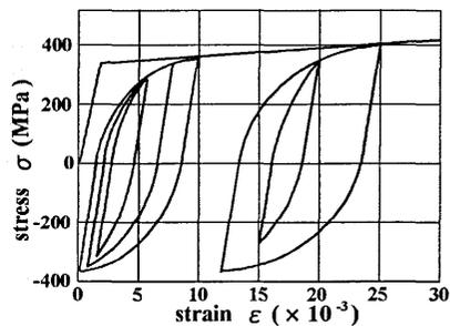
Fig. 8 Steel Material Model [17][18]
