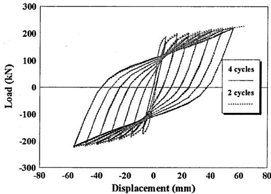
Fig. 11 Load – Displacement Relationship in the Orthogonal Direct. (repeat 4)
