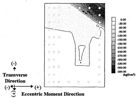
Fig. 18.4 Concrete Stress at  $-2 \delta y (2)$
