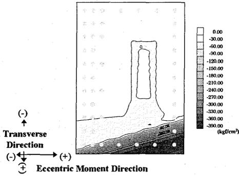
Fig. 18.1 Concrete Stress at  $+2 \delta y (1)$
