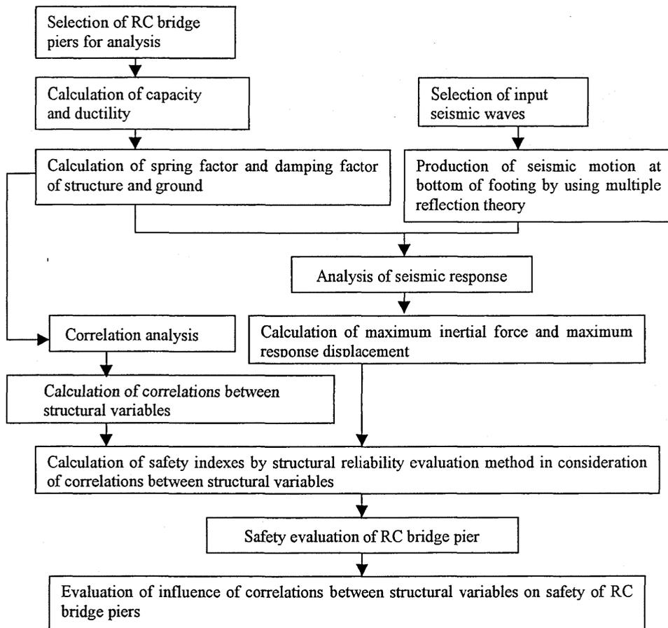
Fig.2 Flow Chart of Seismic Safety Examination for RC Bridge Pier
