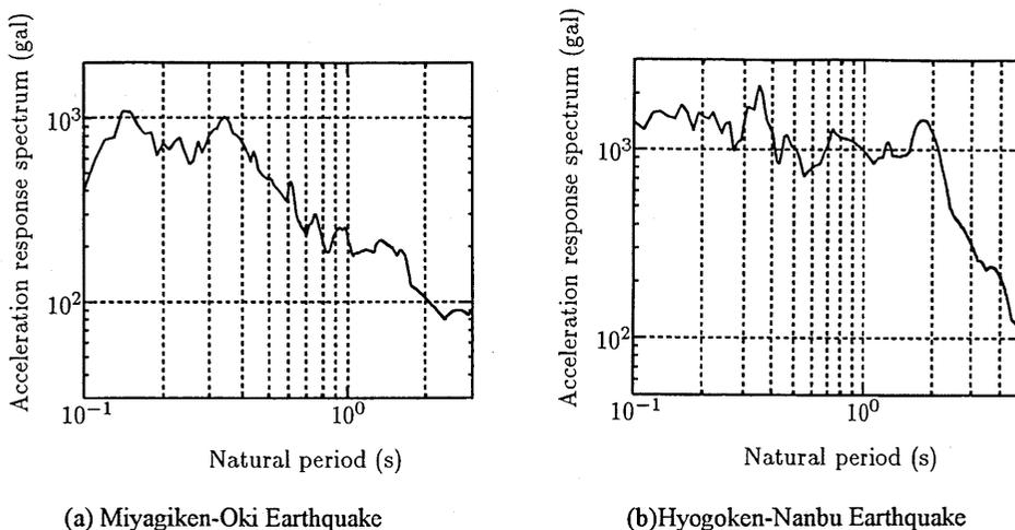
Fig.5 Response Spectrums of Seismic Waveforms at Bedrock in Analysis
