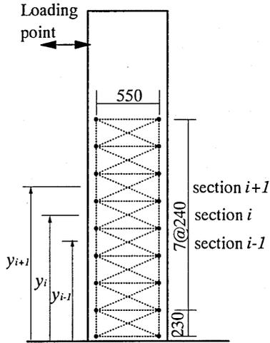
Figure 4 Relative Displacement Measuring Section (unit:mm)
