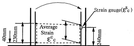
Figure 12 Location of Strain Measurement
