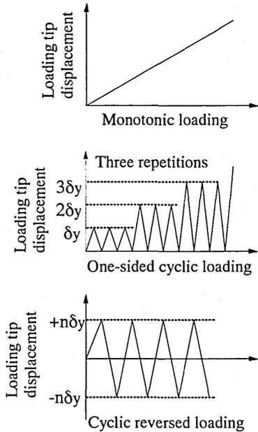
**Figure 3** Loading Procedure
