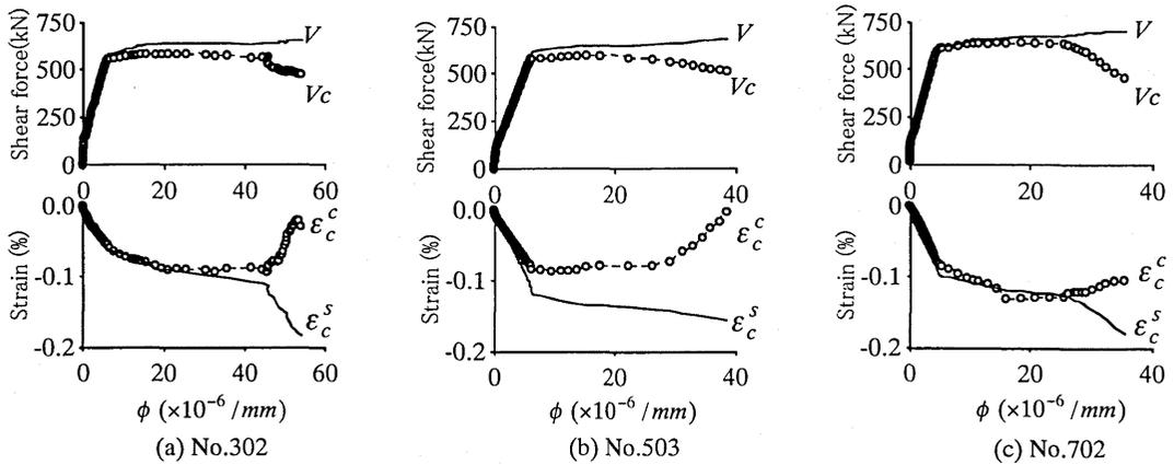
Figure 13 Relationship between  $V_c$  or Compressive Strain and Curvature near Fixed End of Column
