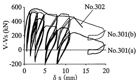
Figure 15 Relationship between Shear Deformation and V-Vs
