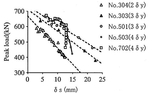
**Figure 8** Relationship between Shear Deformation and Strength Reduction
