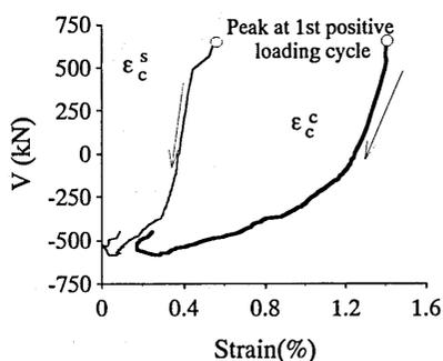
Figure 17 Compressive Strain in 1st Negative Loading Cycle
