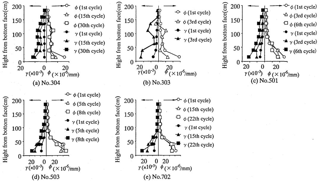
**Figure 9** Curvature and Shear Strain Distribution of Reversed Loaded Specimen
