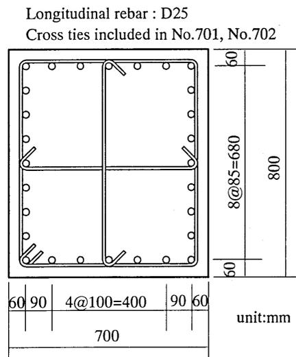
Figure 2 Cross Section of Specimen
