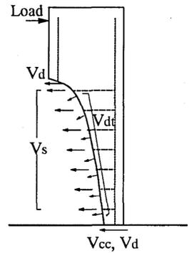
Figure 10 Assumed Shear Resistance Mechanism
