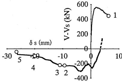
Figure 19 Relationship between  $\delta_s$  and  $V-V_s$  in 1st Cycle of Loading
