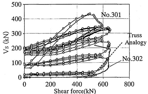
Figure 14 Relationship between Shear Load and  $V_s$
