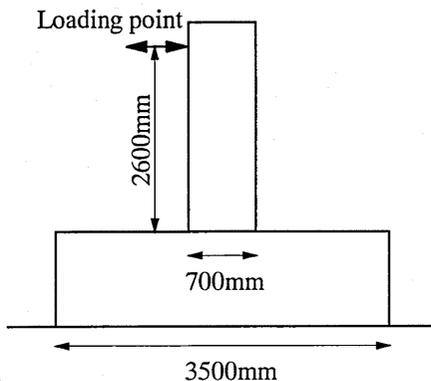
Figure 1 Dimensions of Specimen
