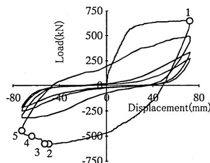
Figure 16 Load-Displacement Hysteresis Loop (No.306)
