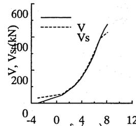
Figure 21 Relationship between Shear Deformation and Load and  $V_s$  (Top:5th cycle loading) (Middle:10th cycle loading) (Bottom:15th cycle loading)
