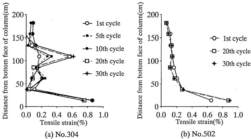
Figure 23 Distribution of Axial Strain
