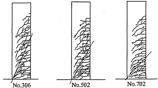
Figure 11 Shear Crack Pattern (at peak of 1st positive loading cycle)
