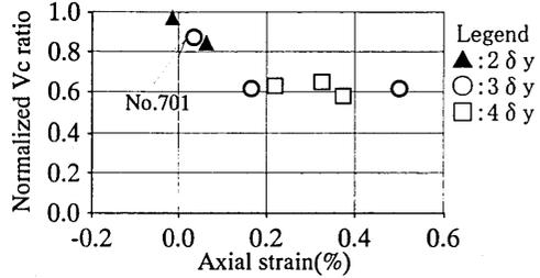
Figure 20 Relationship between Axial Compressive Strain and Normalized  $V_c$  Ratio
