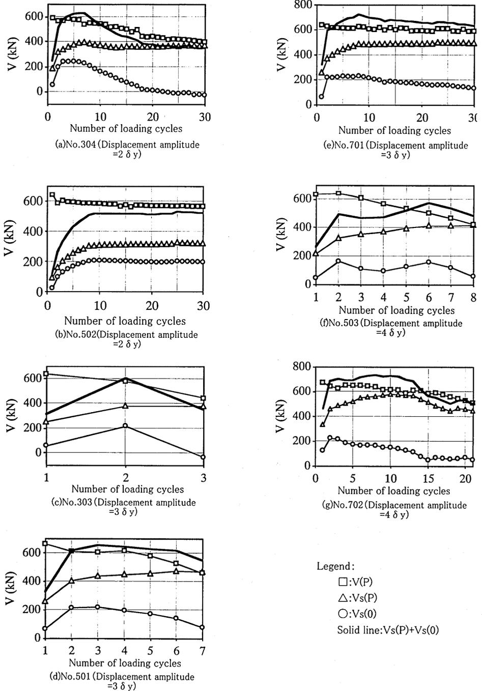
Figure 22 Variation of Vs with Number of Loading Cycles
