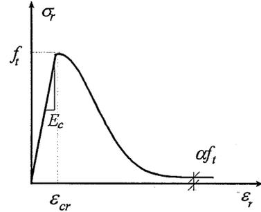
Fig. 3 Tensile stress-strain curve of concrete
