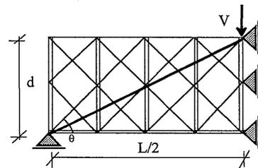
Fig.17 Illustrative beam example (No.2)
