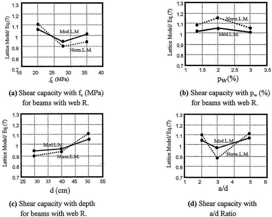
Fig.15 Change of shear carrying capacity for beams with web reinforcement
