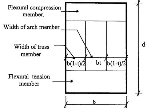
Fig.2 Cross section of concrete beam in the Modified Lattice Model
