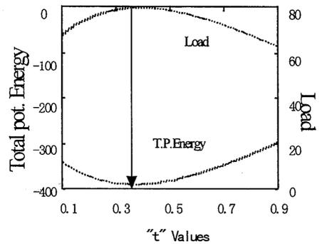
Fig. 6 Behaviour of T.P. energy and applied load for various "t" values
