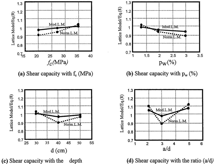
Fig. 16 The change of shear carrying capacity for beams without web reinforcement
