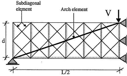
Fig.1 Modified Lattice Model
