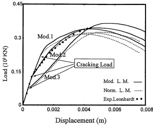
Fig.8 Comparison with experiment (No. 4)
