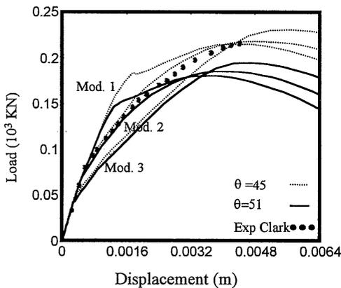
Fig.13 Load-displacement diagram in case of  $\theta=51^\circ$  and  $45^\circ$  (No.2)
