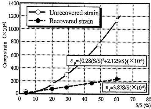
Fig.-8 Relationship between recovered and unrecovered strain
