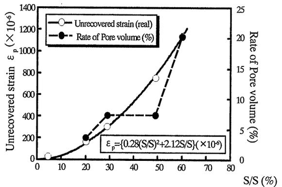
Fig.-10 Unrecovered strain and rate of pore volume
