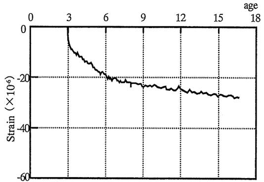
Fig.-6 Strain of unloaded specimen
