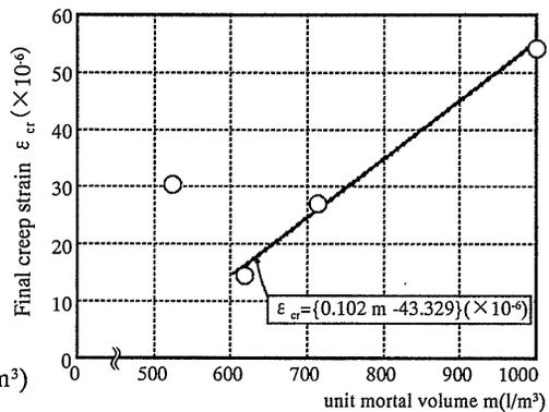
**Fig.-22** Relationship between unit mortal volume and creep strain (tensile creep)
