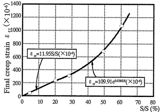
Fig.-7 Relationship between S/S and final creep strain (mortal)
