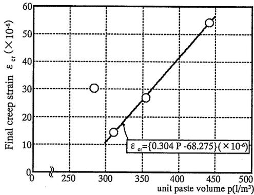
**Fig.-23** Relationship between unit paste volume and creep strain (tensile creep)
