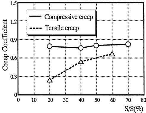
**Fig.-19** Creep Coefficient and S/S of Concrete (loading age was 5 days)
