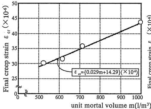
**Fig.-20** Relationship between unit mortal volume and creep strain (compressive creep)
