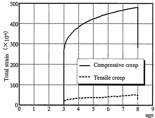
Fig.-13 Creep strain (Mortal at  $S/S=20\%$ )
