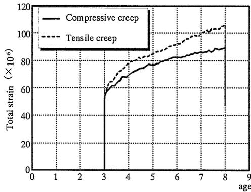
Fig.-11 Total strain (Mortal at  $1\text{N/mm}^2$ )
