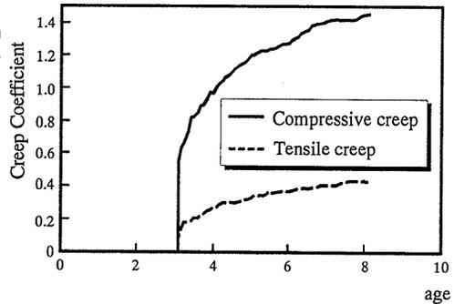
**Fig.-17** Creep Coefficient (Concrete at 1N/mm<sup>2</sup>)
