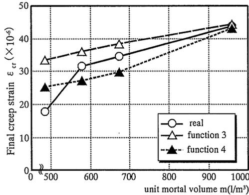
**Fig.-26** Calculated creep strain
