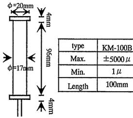
Fig.-1 Embedded strain meter
