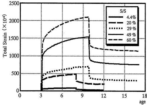
Fig.-5 Change of total strain (mortal)
