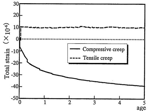
**Fig.-24** Creep of Coarse aggregate
