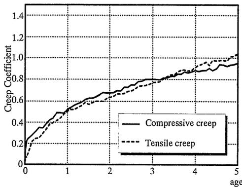
Fig.-12 Creep Coefficient (Mortal at  $1\text{N/mm}^2$ )
