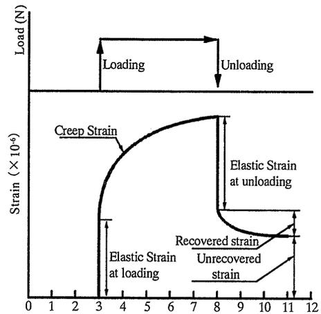
Fig.-4 Loading pattern and strain
