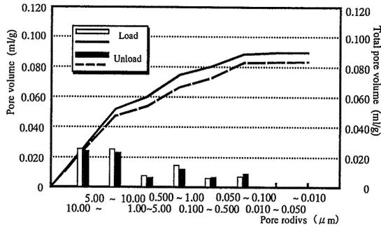
**Fig.-15** Pore size distribution of tensile creep
