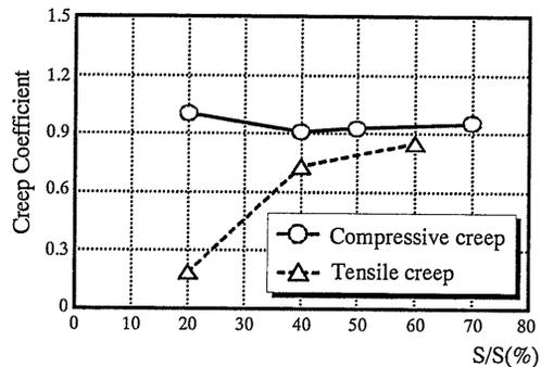
**Fig.-18** Creep Coefficient and S/S of Concrete (Loading age was 3 days)
