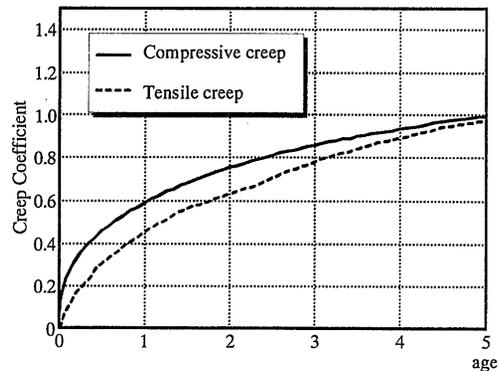
Fig.-14 Creep Coefficient (Mortal at  $S/S=20\%$ )
