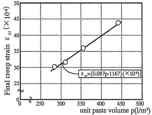
**Fig.-21** Relationship between unit paste volume and creep strain (compressive creep)
