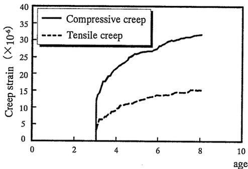
**Fig.-16** Creep strain (Concrete at 1N/mm<sup>2</sup>)
