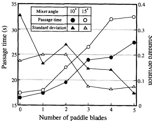
**Fig.22** Relationship between number of paddle blades and passage time and standard deviation
