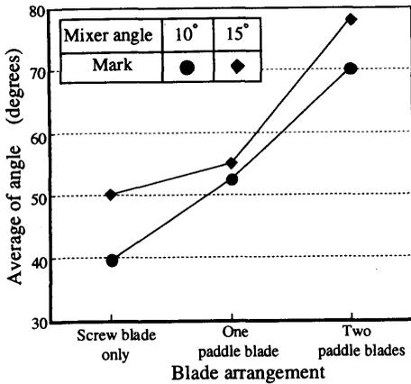
Fig.7 Average angle by blade arrangement
