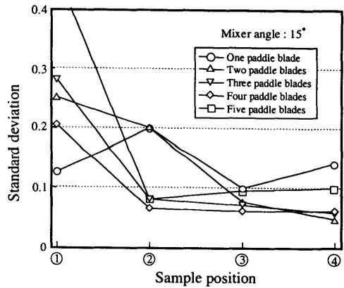
**Fig.21** Standard deviation from initial value  $Vg/Vm=0.4$  (mixer angle  $15^\circ$ )
