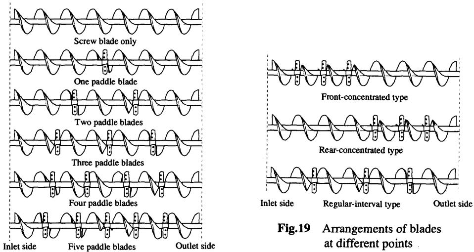
**Fig.19** Arrangements of blades at different points
