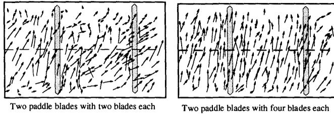
Fig.10 Velocity vector distribution of tracer by shape of paddle blades
