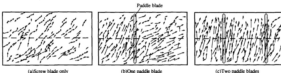
**Fig.5** Velocity vector distribution of tracer by blade arrangement
