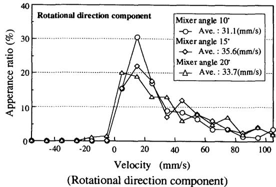
**Fig.16** Velocity distribution of each component by mixer angle
