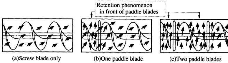
Fig.9 Notion of partial retention phenomenon by paddle blades
