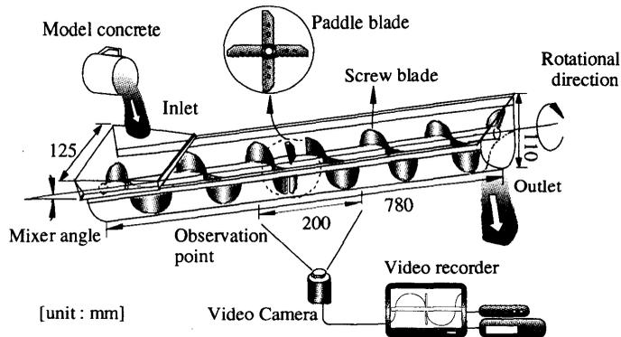
Fig.1 Illustration of model continuous mixer
