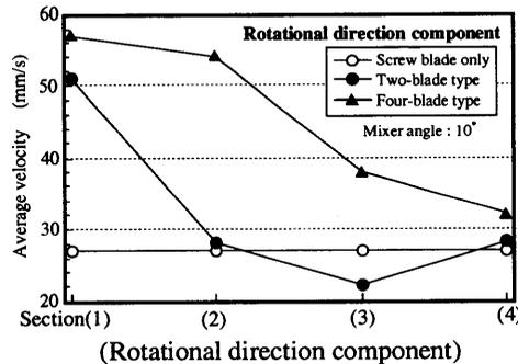
Fig.14 Average velocity of each section by shape of paddle blade
