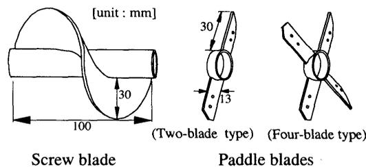
Fig. 2 Types of blades used in continuous mixer
