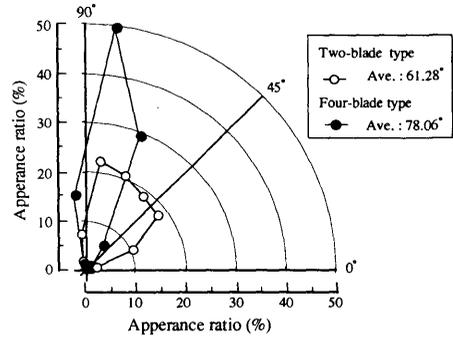
Fig.11 Appearance ratio of vector angle by shape of paddle blade
