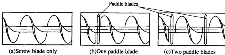
**Fig.3** Arrangements of blades at observation point
