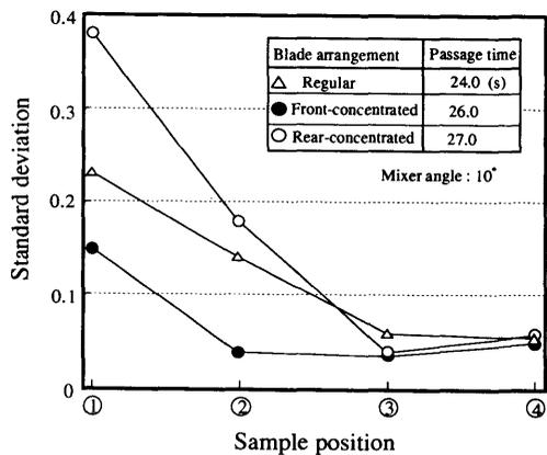
**Fig.23** Standard deviation from initial value  $Vg/Vm=0.4$  (three paddle blades)
