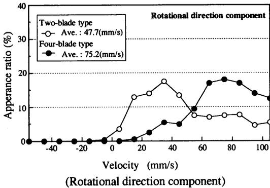
Fig.12 Velocity distribution of each component by shape of paddle blade
