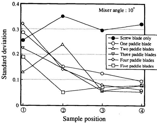
**Fig.20** Standard deviation from initial value  $Vg/Vm=0.4$  (mixer angle  $10^\circ$ )
