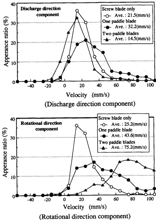
Fig.8 Velocity distribution of each component by blade arrangement
