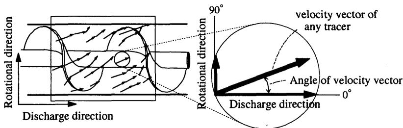
**Fig.4** Angle and components of velocity vector
