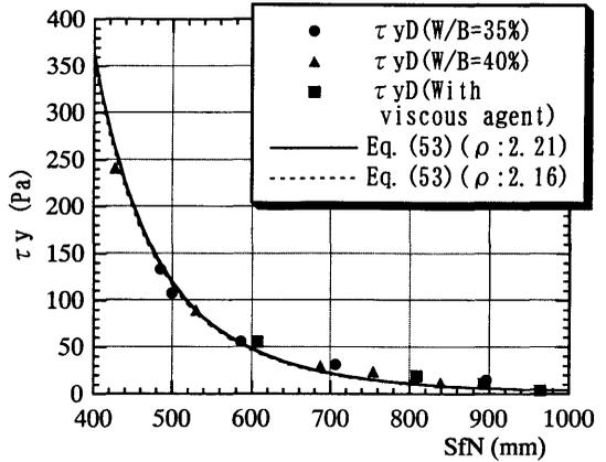
**Fig. 11** Relationship between normalized slump flow and yield value
