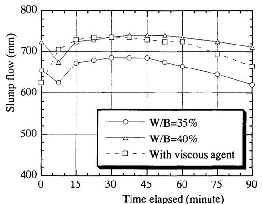
**Fig. 2** Changes in slump flow with time
