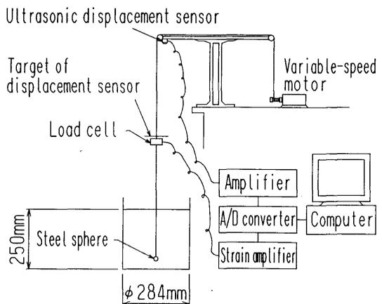
Fig.3 Sphere drag viscometer
