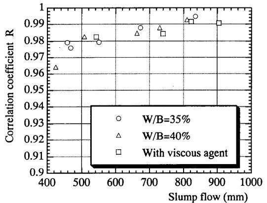
**Fig. 6** Relationship between slump flow and correlation coefficient
