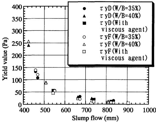
**Fig. 10** Relationship between slump flow and yield value
