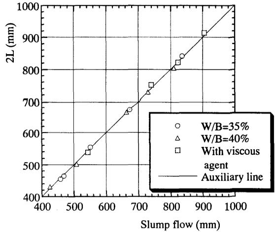
**Fig. 8** Comparison between slump flow and  $2L$
