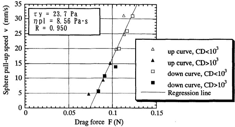
Fig. 4 Example of sphere drag test result
