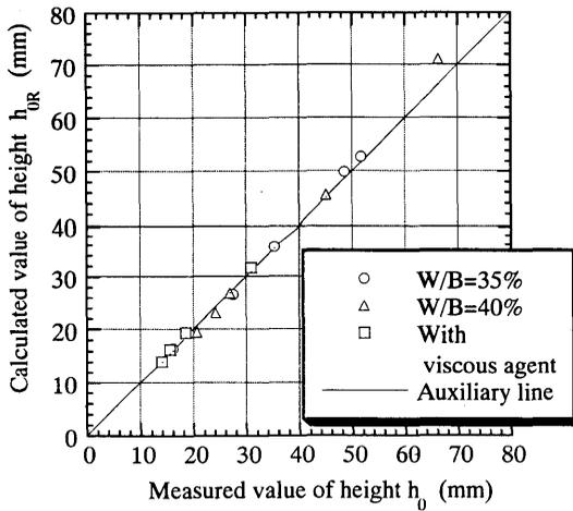
**Fig. 7** Comparison between measured and calculated values of height of center of specimen
