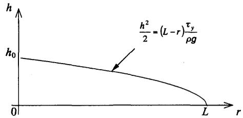
**Fig.1** Height distribution of specimen derived from theoretical equation (38)
