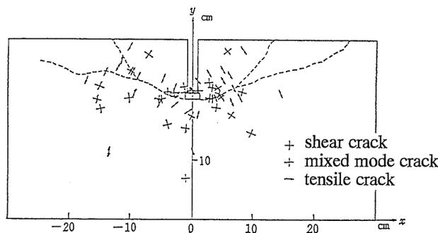
Fig. 9 Moment tensor analysis in a pull-out test.
