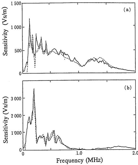
Fig. 4 Frequency response of AE sensors
