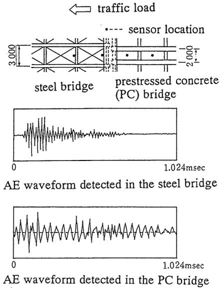
Fig. 14 AE waveforms detected in a composite bridge
