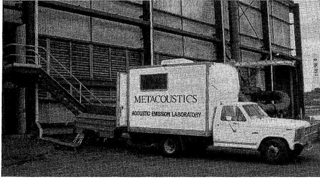
Photo 1 A mobile facility for AE measurement
