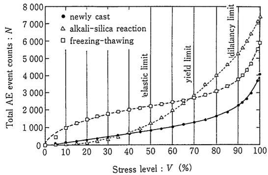
Fig. 13 Total AE event count versus stress level in concrete sample
