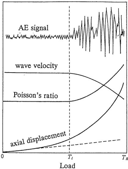
Fig. 1 Mechanical parameters of concrete under compression [7]
