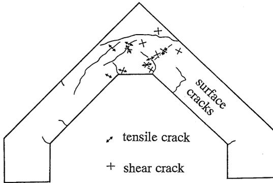
Fig. 15 Moment tensor analysis in a tensile test of an RC frame
