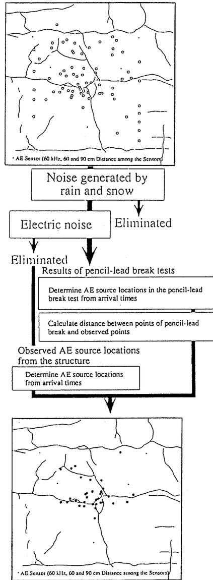
Fig. 16 Two-dimensional source location in a concrete retaining wall
