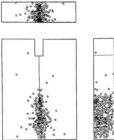
Fig. 12 Identification of the fracture process zone by AE source location
