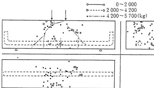
(b) AE locations subjected to diagonal shear failure
