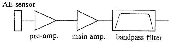
Fig. 3 AE measuring system
