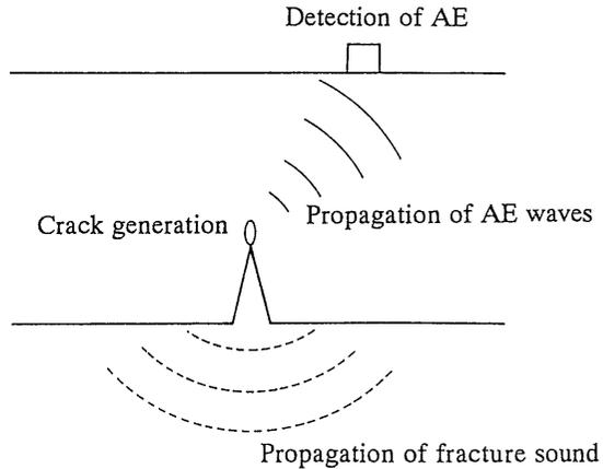
Fig. 2 Generation, propagation and detection of AE signals
