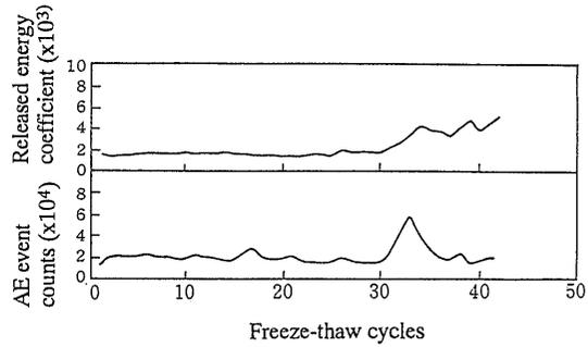
Fig. 11 AE generation during freeze-thaw action
