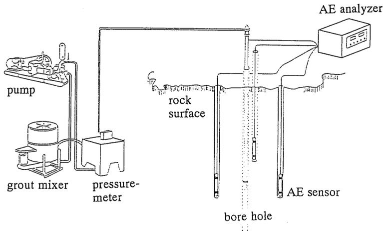
Fig. 17 AE monitoring system for grouting
