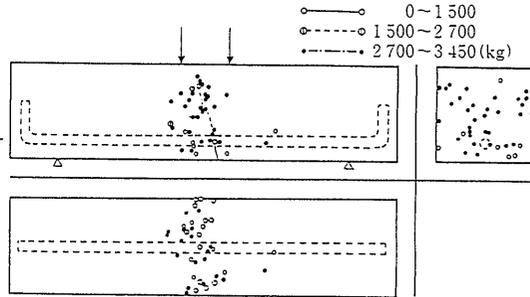
(a) AE locations subjected to bending failure
