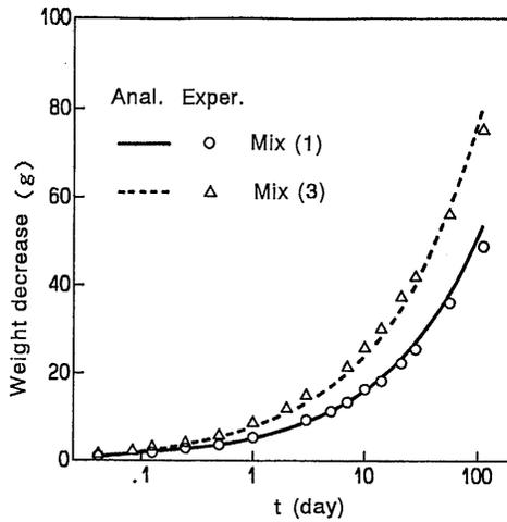
**Fig.12** Weight decrease for one-face drying
