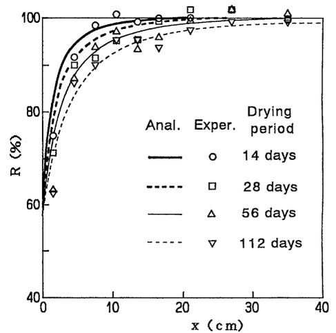
**Fig.11** Profiles of relative water content for one-face drying
