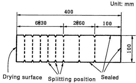
**Fig.1** One-face drying specimen
