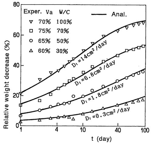
**Fig.13** Weight decrease for six-face drying
