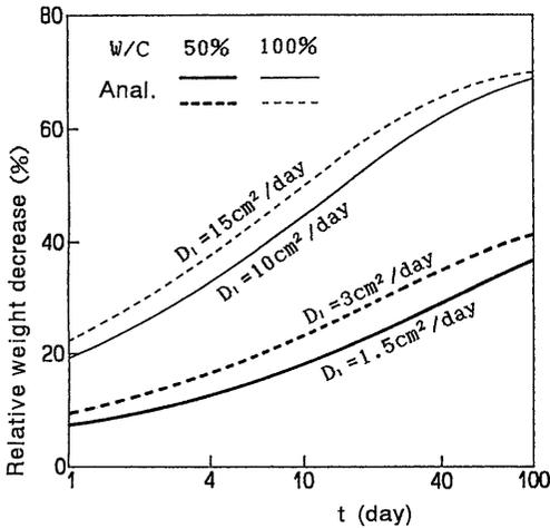
**Fig.10** Dependence of weight decrease on  $D_1$  for six-face drying
