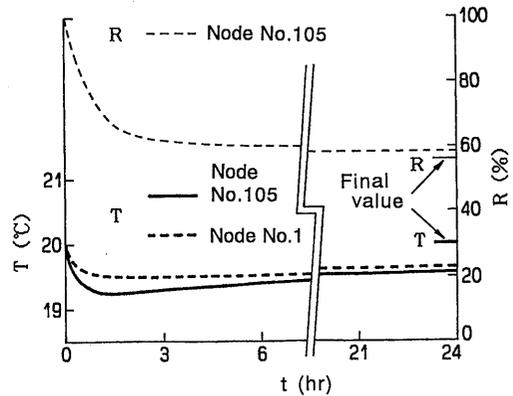
**Fig.6** Temperature and relative water content at drying surface
