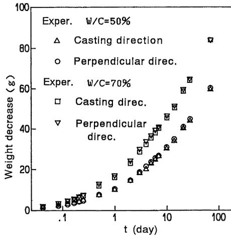
Fig.7 Weight decrease for direction of drying
