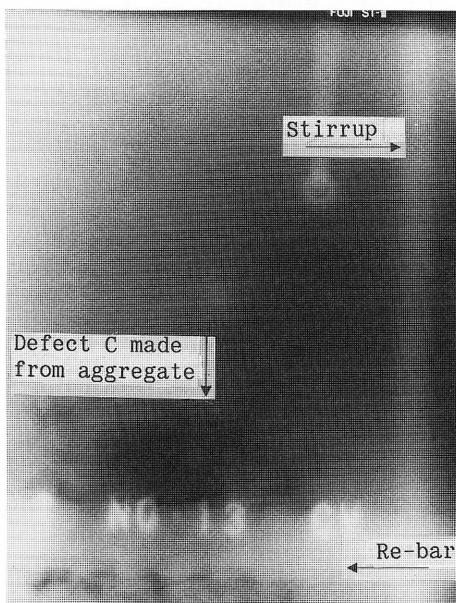
Photo.2 Radiograph of zone with defect C after increasing the light intensity
