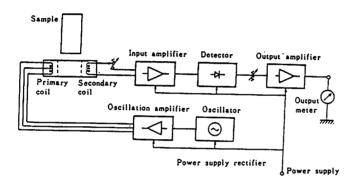
Fig. 1 Example of magnetic probing apparatus
