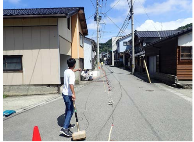
Fig.7 SWS measurement situation at Line B (moving source measurement)
