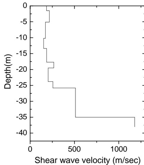
**Fig.10** PS logging (S wave velocity profile) (Shear wave distribution along the depth at station 40)
