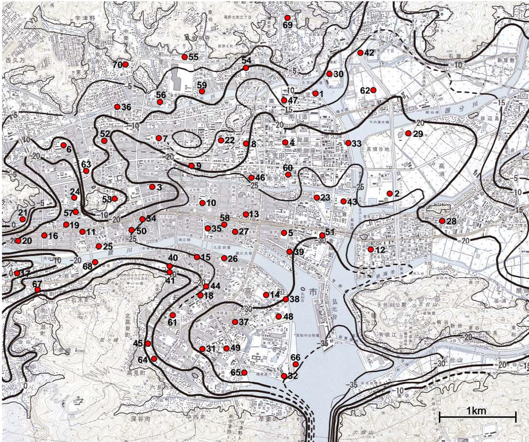
**Fig.6** Microtremor Observation Stations Topographical map issued by GSI was used. Contour (bottom of alluvial layer, unit for contours in meters) was added referring “The Ground Diagram of Kochi<sup>11)</sup>”
