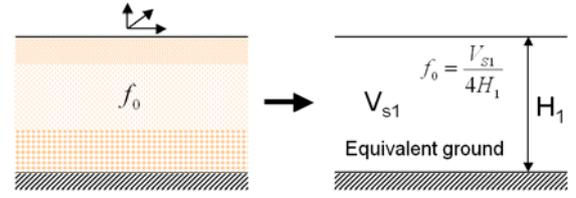
**Fig.4** Replacement of multi-layer ground with an equivalent homogeneous ground
