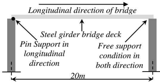
**Fig.3** End condition of selected span of target highway
