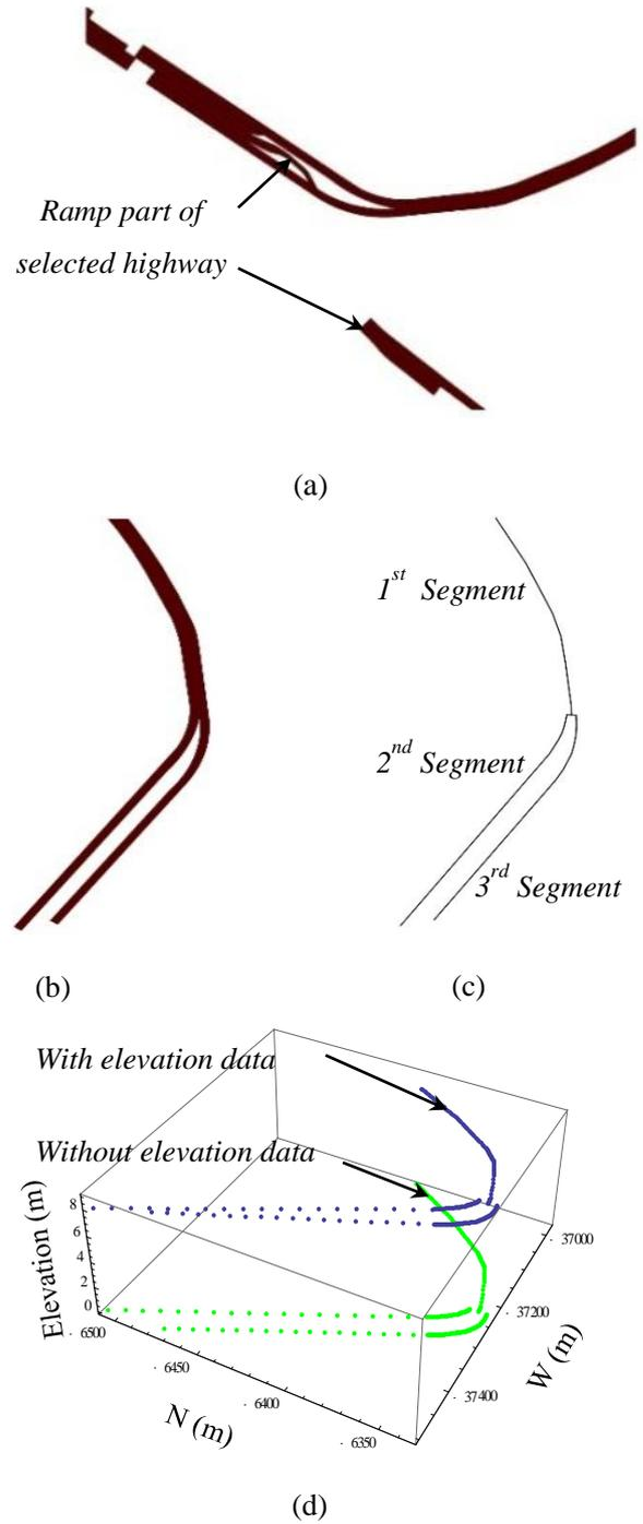
**Fig.2** Example of applying decoding procedures to GIS data: (a) exclusion of highway main-class tunnel sub-class; (b) exclusion of highway main-class tunnel and ramp part; (c) extraction of 2D centre line arrangement; and (d) arrangement of 3D centre line.
