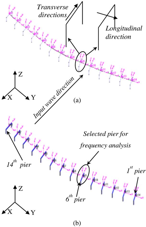
**Fig.4** CAD model for selected highway segment: (a) frame CAD model; and (b) solid CAD model
