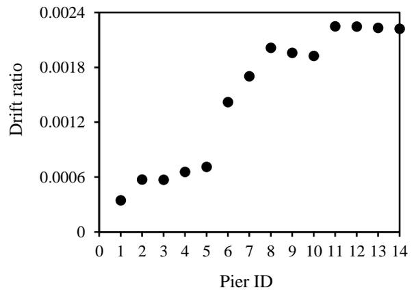
**Fig.7** Drift ratio in each pier along local X-axis of pier.
