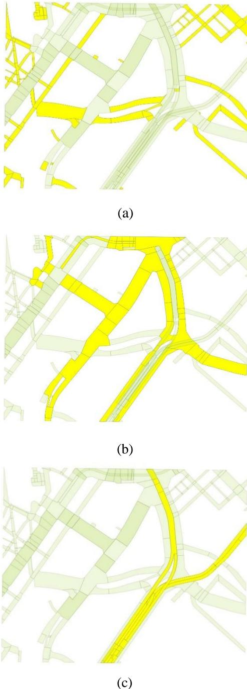
**Fig.1** Example of decoding of GIS data to identify network configuration: (a) decoded configuration; (b) extraction of main local road; and (c) extraction of highway.
