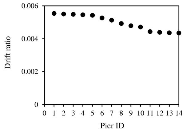
**Fig.8** Drift ratio in each pier along local Y-axis of pier.
