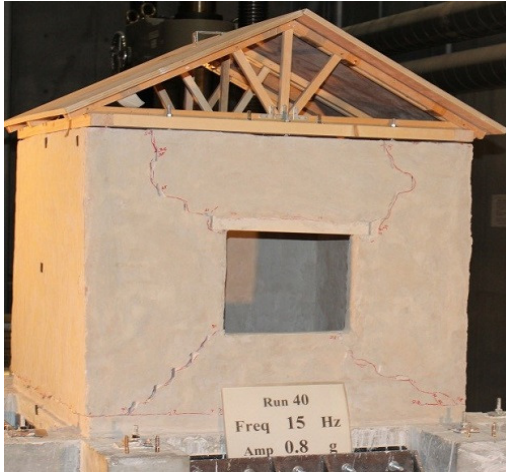
Fig.10 URM house at Run-40 15 Hz and 0.8g
