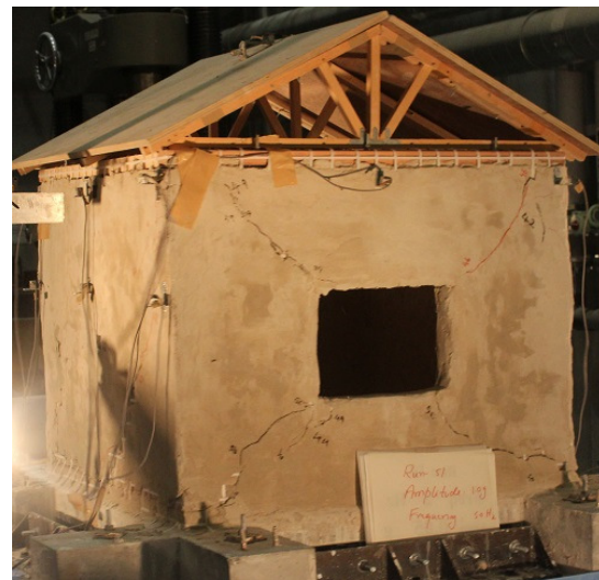
Fig.12 PPN house at Run-51 5 Hz and 1.0g
