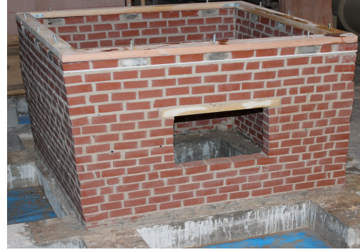
Fig.2 Model House after completion of brick work then connected with out of plane connection. The vertical Piece was attached at pitch of 50 mm with bottom piece of PP-band as shown in Fig.4.
