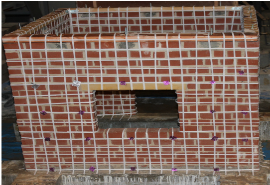
Fig.8 Non Connected PP-band house (PPN)
