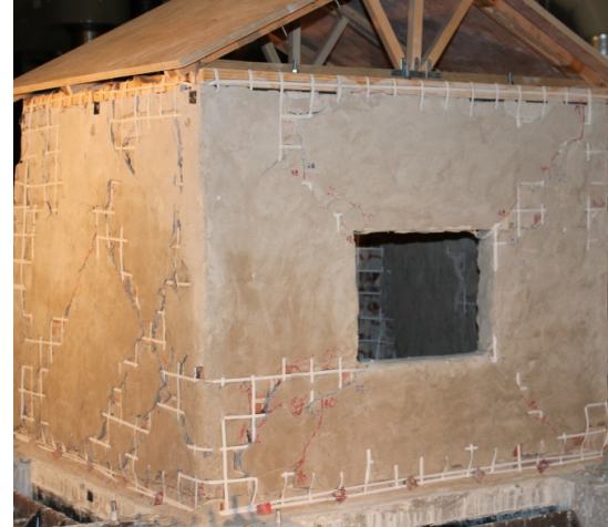
Fig.11 PPF house at Run-50 2 Hz and 0.8g
