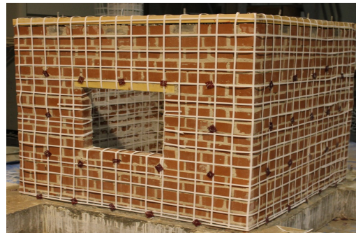
Fig.5 Fully Connected PP-band house (PPF)
