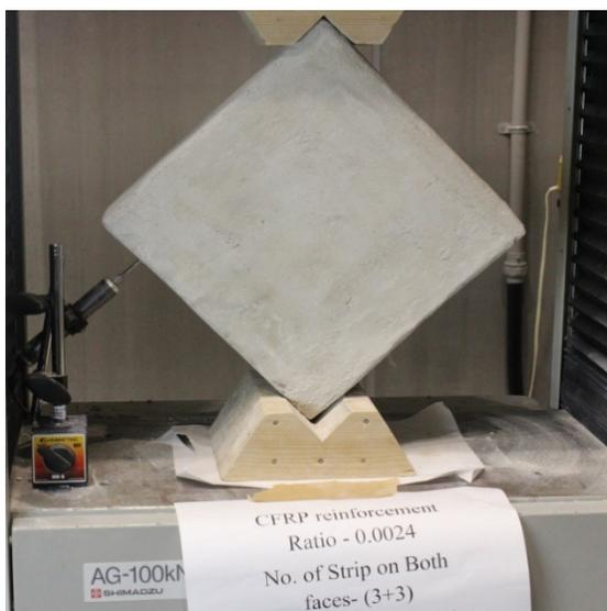
Fig.3 Test setup of masonry wallet under diagonal compression.
