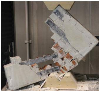
(c) Failure pattern of masonry wallet retrofitted with 0.0072 CFRP volumetric ratio with four strips on each face.
