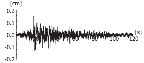
Fig.14 Low cut component (more than 0.2[Hz]) of the error of integration ( Cut off frequency : 0.2[Hz], Big amplitude ) .
