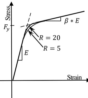
**Figure 3** Stress strain model for steel02<sup>15, 16</sup>
