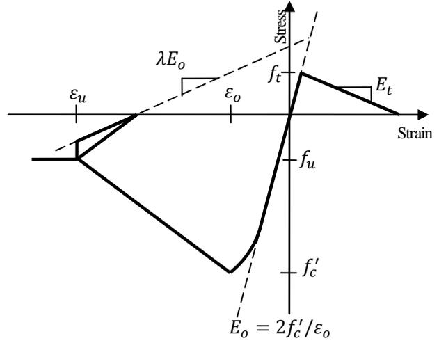
**Figure 2** Stress strain model for concrete Concrete02<sup>15</sup>
