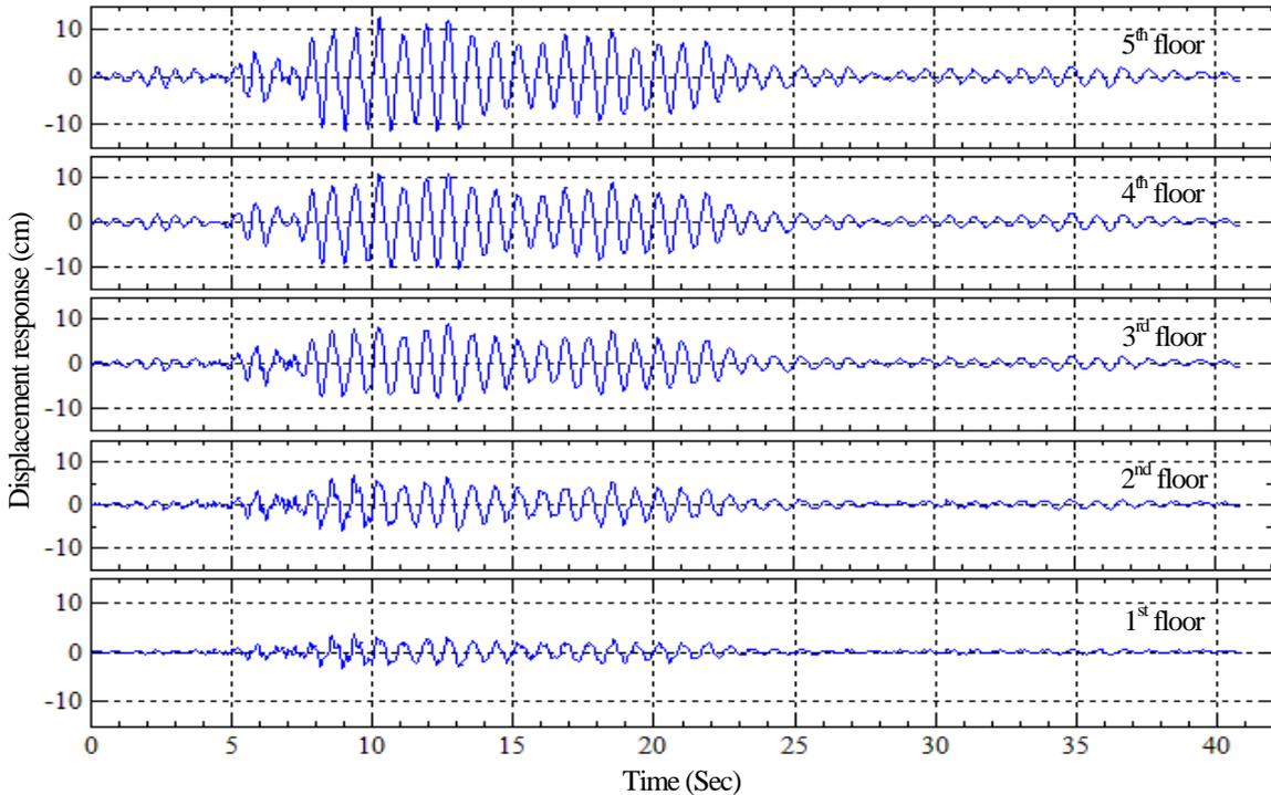
**Figure 4** Displacement response of concrete frame against a random GM out of set of possible GMs
