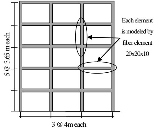
Figure 1 Elevation of concrete frame
