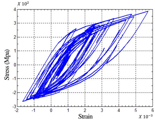
**Figure 5** Stress strain response of steel fiber of ground floor column at maximum stressed section
