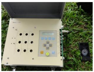
Figure 5. GPL-6A3P Portable Receiver - Microtremor Device
