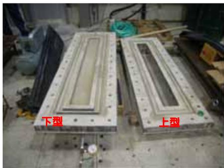
(a) 止水実験型枠
